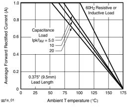
Figure 1. Forward Current Derating Curve
