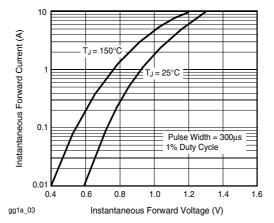
Figure 3. Typical Instantaneous Forward Characteristics
