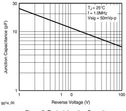
Figure 5. Typical Junction Capacitance
