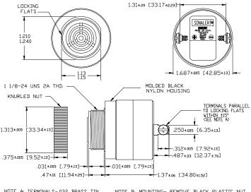
NOTE A: TERMINALS-.032 BRASS TIN PLATED, TAPPED FOR #6-32 SCREW. TWO #6-32 NICKEL PLATED BRASS SCREWS INCLUDED. WILL ACCEPT 1/4\* QUICK CONNECT. NOTE B: MOUNTING- REMOVE BLACK PLASTIC NUT AND INSERT THREADED FRINT THROUGH 1.25' HOLE PUNCHED IN PANEL, IF DRIENTATION IS NEEDED, NOTE LOCKING FLATS ON DRAVING. SCREW NUT BACK ON. DO NOT DVERTIGHTEN.
