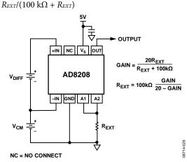
Figure 30. Adjusting for Gains Less than 20
