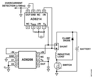
Figure 27. Battery-Referenced Shunt Resistor
