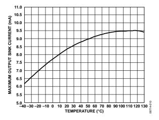
Figure 10. Maximum Output Sink Current vs. Temperature
