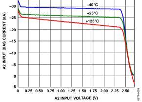
Figure 9. Input Bias Current of A2 vs. Input Voltage and Temperature
