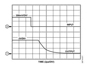
Figure 17. Differential Overload Recovery, Falling
