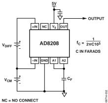
Figure 33. Single-Pole, Low-Pass Filter Using the Internal 100 k $\Omega$  Resistor
