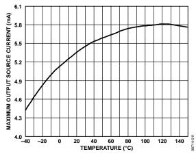
Figure 11. Maximum Output Source Current vs. Temperature
