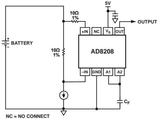
Figure 29. 4 mA to 20 mA Current Loop Receiver
