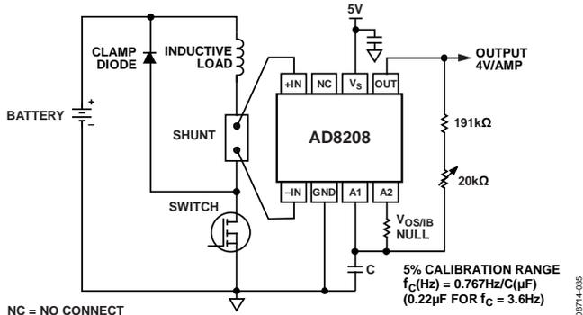
Figure 36. High Line Current-Sensor Interface;
