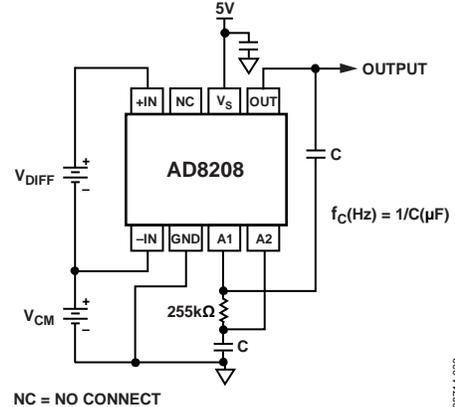
Figure 34. Two-Pole, Low-Pass Filter
