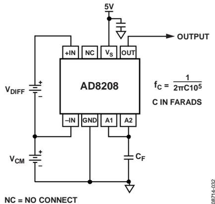
Figure 33. Single-Pole, Low-Pass Filter Using the Internal 100 kΩ Resistor
