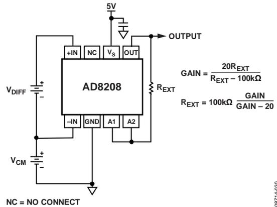
Figure 31. Adjusting for Gains Greater than 20
