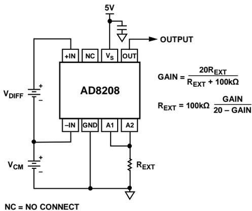
Figure 30. Adjusting for Gains Less than 20
