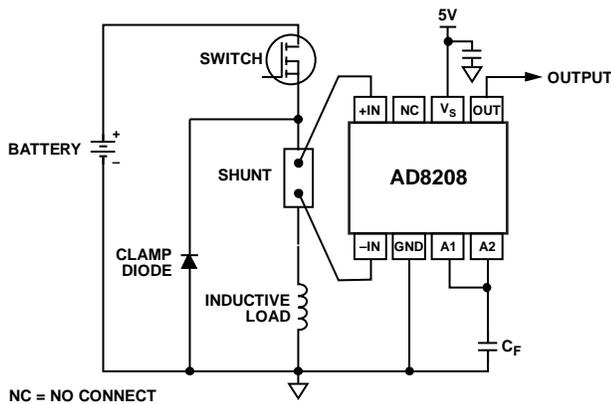
Figure 26. High-Side Switch
