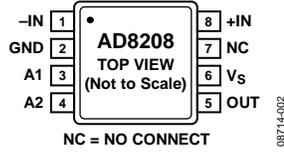
Figure 2. Pin Configuration
