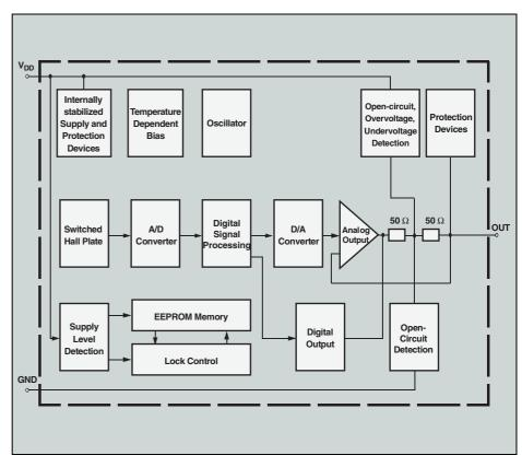
Fig. 2: Block diagram of the HAL 83x
