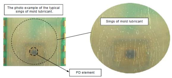
The ruggedness on the surface of the resin seen in the photograph above is the signs of the mold lubricant, not scratches.
