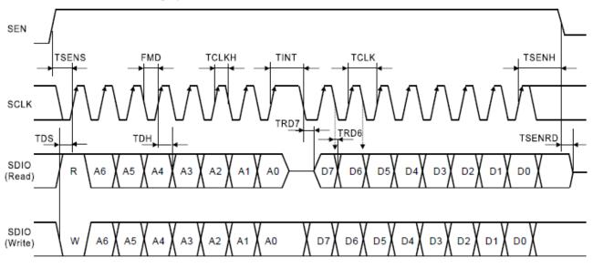
Figure Serial interface protocol (Register write & read)
