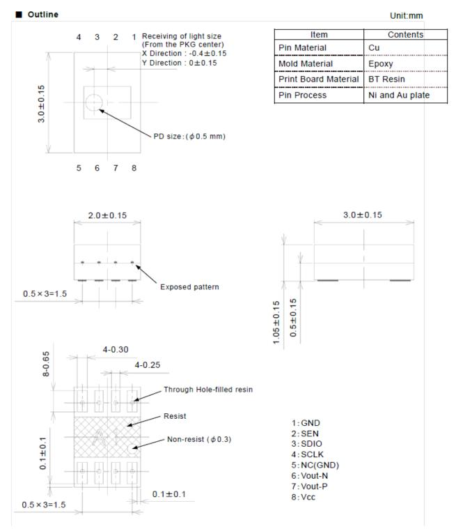
(Note1) Dimension tolerance without instructions should be ±0.075 mm.
