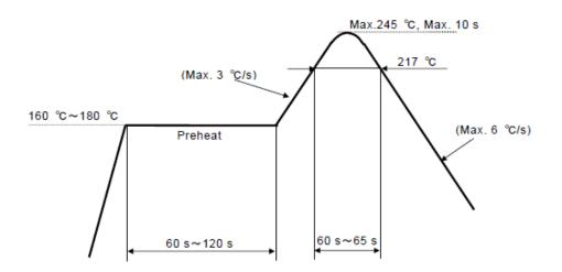
(Soldering time : Maximum 1 time) It is temperature profile at surface of printed board.
