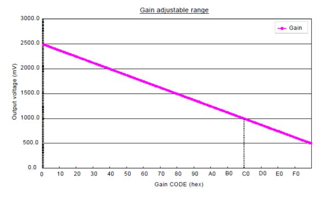
The gain can be adjusted within the range of +7.8 dB from -6 dB based on BFh (0 dB). Vertical axis is plotted Gain. This chart shows that Vout-P-Vout-N is 1V at BFh.
