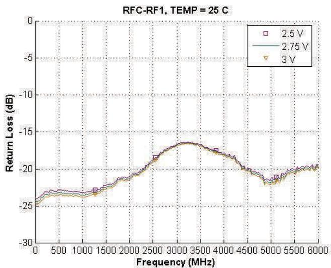
Figure 16. Return Loss: RF1 @ 2.75V (RFC-RF1 Active Path)
