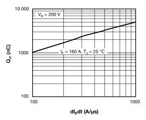
Fig. 7 - Typical Reverse Recovery Charge vs. dl<sub>F</sub>/dt (Per Leg)
