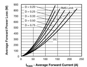
Fig. 5 - Forward Power Loss Characteristics
