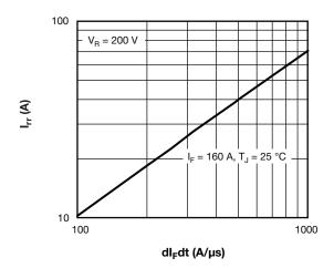
Fig. 8 - Typical Reverse Recovery Current vs. dl<sub>F</sub>/dt (Per Leg)
