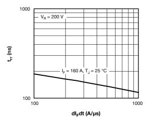
Fig. 6 - Typical Reverse Recovery Time vs. dl<sub>F</sub>/dt (Per Leg)
