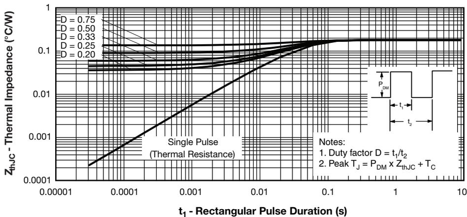
Fig. 4 - Maximum Thermal Impedance  $Z_{thJC}$  Characteristics
