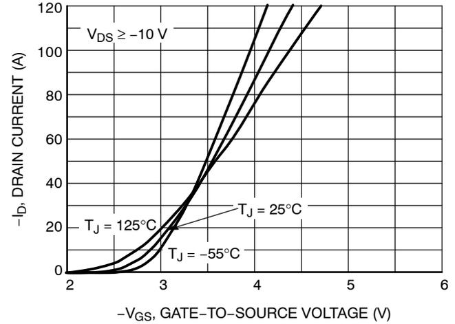
Figure 2. Transfer Characteristics
