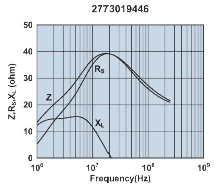
Impedance, reactance, and resistance vs. frequency.
