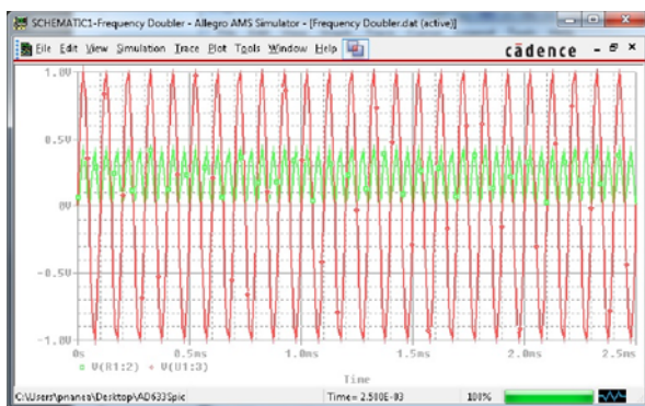
Figure 33. Frequency Doubler Response Graph Displayed in PSPICE
