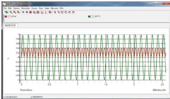
Figure 39. Frequency Doubler Response Graph Displayed in SIMetrix
