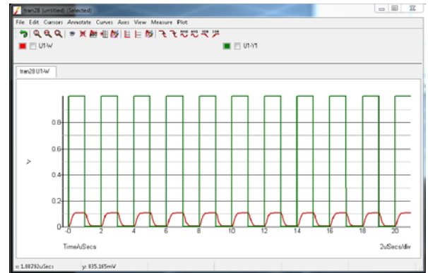
Figure 41. Pulse Circuit Response Displayed in SIMetrix
