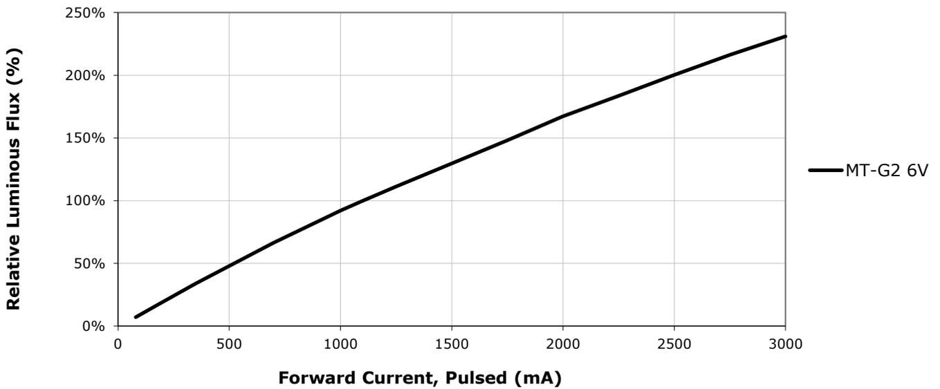
RELATIVE LUMINOUS FLUX VS. CURRENT ( $T_j = 85\text{ }^\circ\text{C}$ ) - CONTINUED
