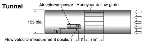
Measurement conditions: Power supply voltage of 12 VDC and ambient temperature of 25°C
