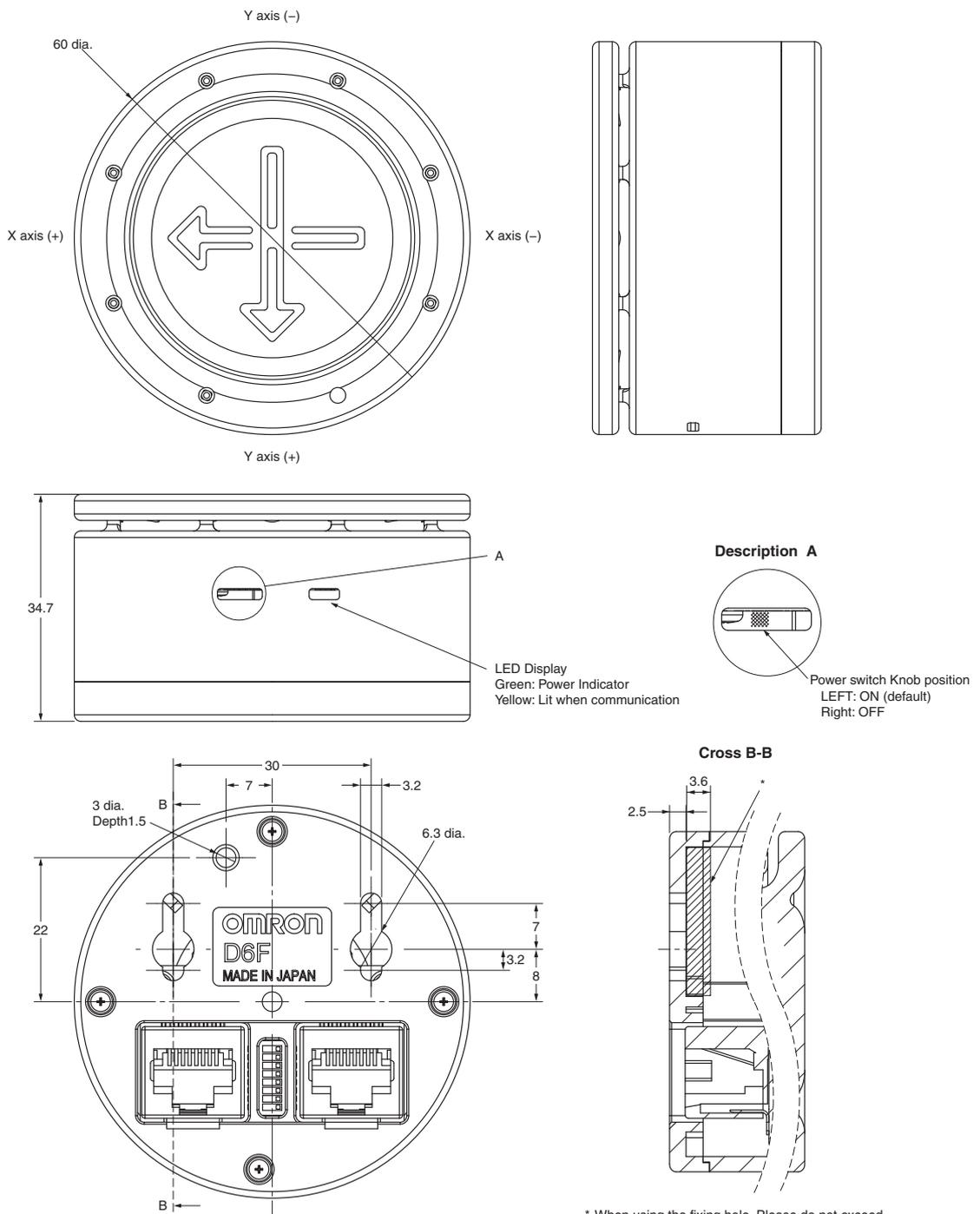
\* When using the fixing hole, Please do not exceed the depth (3.6 mm) of the shaded portion.
