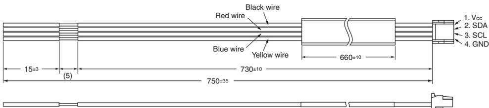
Contact :SSHL-002T-P0.2 (Manufactured by J.S.T. Mfg. Co., Ltd.)
