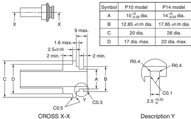
Note. There is a possibility that leak damage or faulty of the body occurs when static load of more than 40 N is applied to 300 mm from the center of product as fulcrum point.
