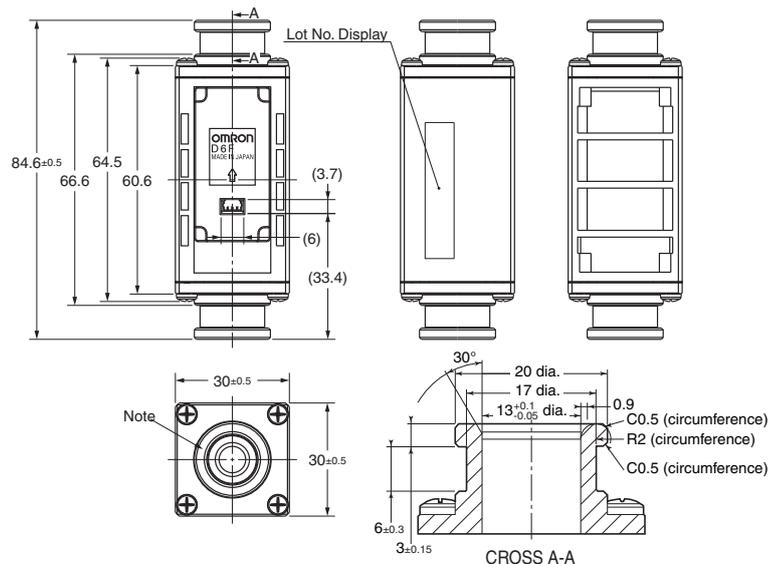
Note. The Port type of pipe fitting based on "Quick Joint P10 Type".
