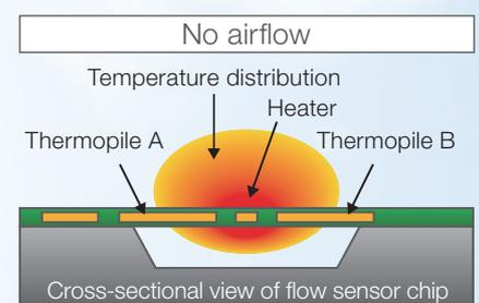
During the absence of airflow, the temperature distribution around the heater is symmetrical. When there is airflow, the temperature of the upwind side cools down and the temperature of the downwind side warms up, disrupting the symmetry of the temperature distribution.
