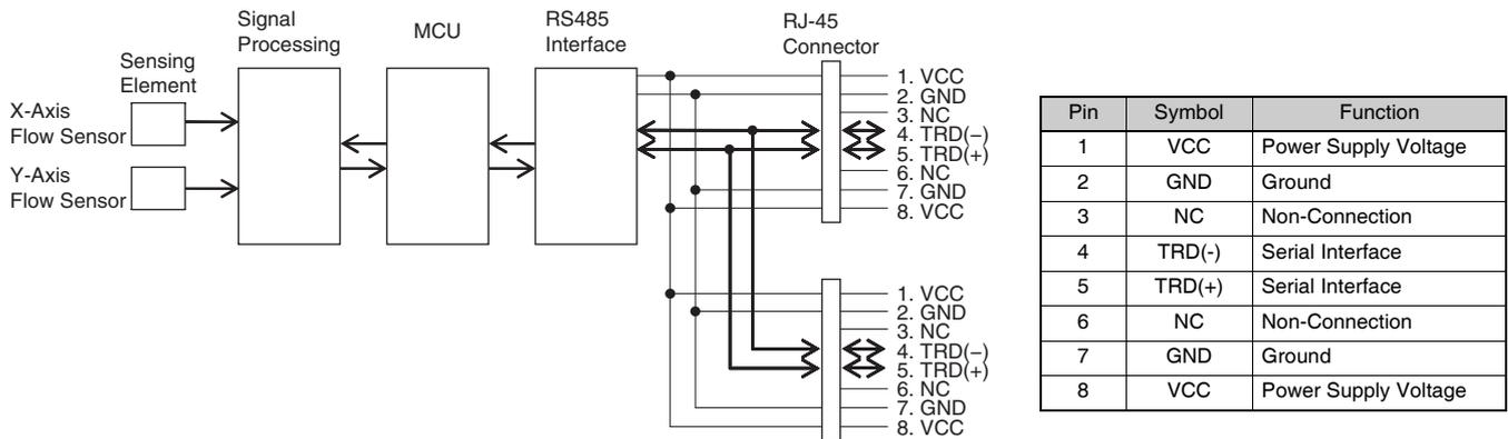
The sensor has two port of RJ-45 connectors (8 pins), and all the pair of each pin is connected internally. These connectors can be used for daisy chain wiring when using multiple devices on the same bus (multi-drop connection).
