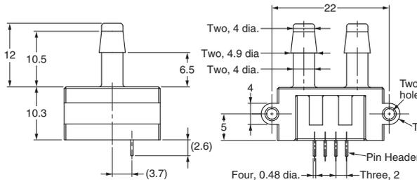
**Recommendation size for pin header installation (tolerances:  $\pm 0.1$ )**
