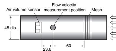
Measurement conditions: Power supply voltage of 3.3 VDC, ambient temperature of 25°C, and dry air.
