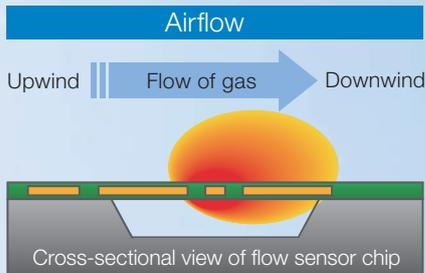
By detecting this temperature difference appearing as a difference in the electromotive forces developed by the thermopiles, it allows the mass flow rate and mass flow velocity to be measured without the influence of temperature and pressure. Since the thermopile generates the thermo-electromotive force, the power consumption is much lower than when using the resistivity method.
