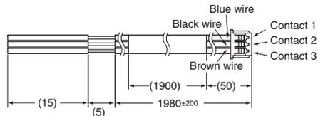
Contact :SZH-002T-P0.5 (Manufactured by J.S.T. Mfg. Co., Ltd.)
