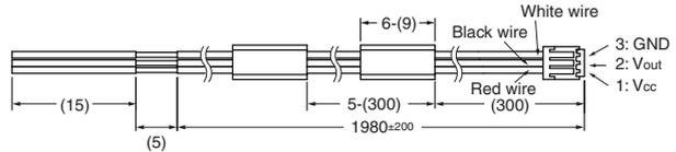
Contact :SSH-003T-P0.2 (Manufactured by J.S.T. Mfg. Co., Ltd.)
