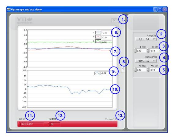
Figure 2. SCC1300 Demo Kit Graphical User Interface
