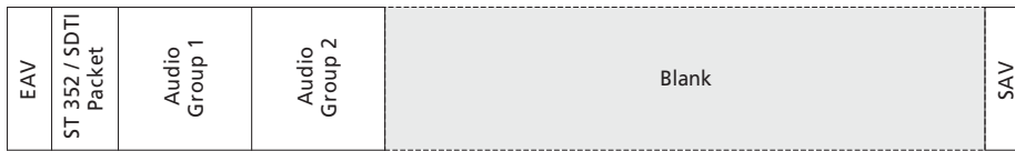
Correct placement of Ancillary Data within HANC Space
