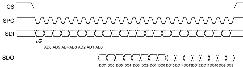
**SPI write****Figure 10. SPI write protocol (in mode 3)**
