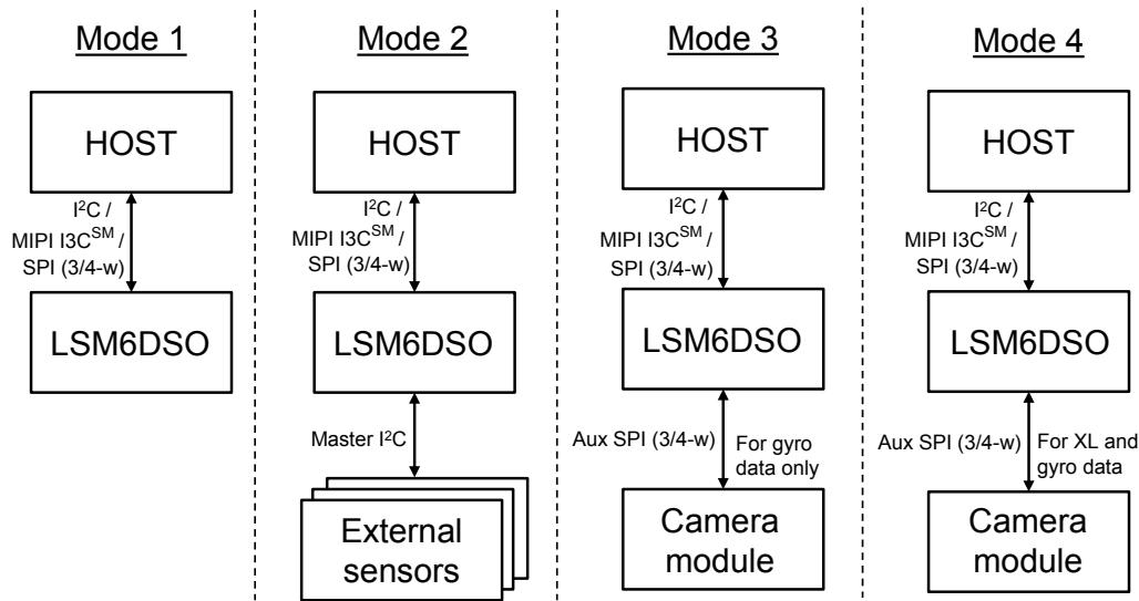
In the following table each mode is described for the pin connections and function.
