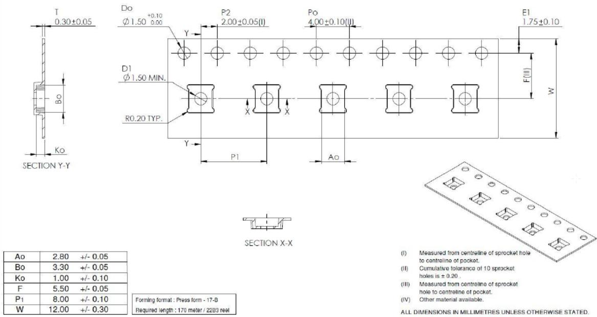
**Figure 27. LGA-14 package orientation in carrier tape**
