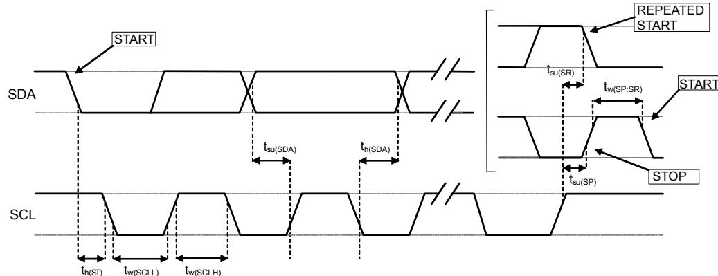
Note: Measurement points are done at  $0.2 \cdot Vdd\_IO$  and  $0.8 \cdot Vdd\_IO$  for both ports.
