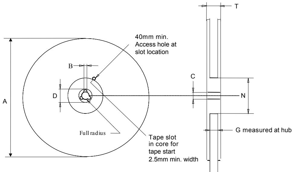
Table 389. Reel dimensions for carrier tape of LGA-14 package
