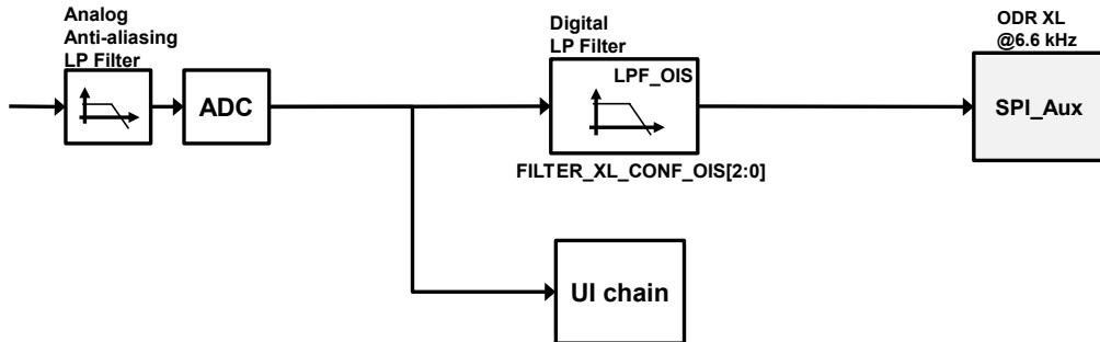
Note: Mode 4 is enabled when Mode4\_EN = 1 and OIS\_EN\_SPI2 = 1 in CTRL1\_OIS (70h).
