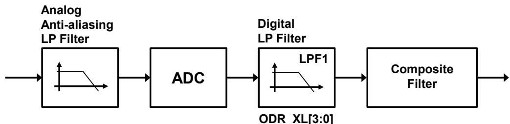
**Figure 17.** Accelerometer composite filter
