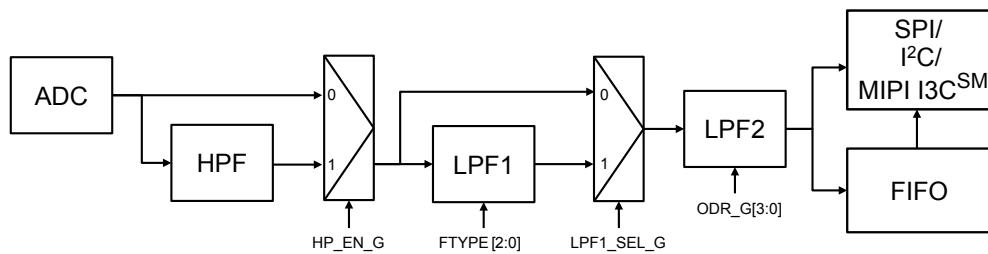
In this configuration, the gyroscope ODR is selectable from 12.5 Hz up to 6.66 kHz. A low-pass filter (LPF1) is available if the auxiliary SPI is disabled, for more details about the filter characteristics see [Table 60. Gyroscope LPF1 bandwidth selection](#).
