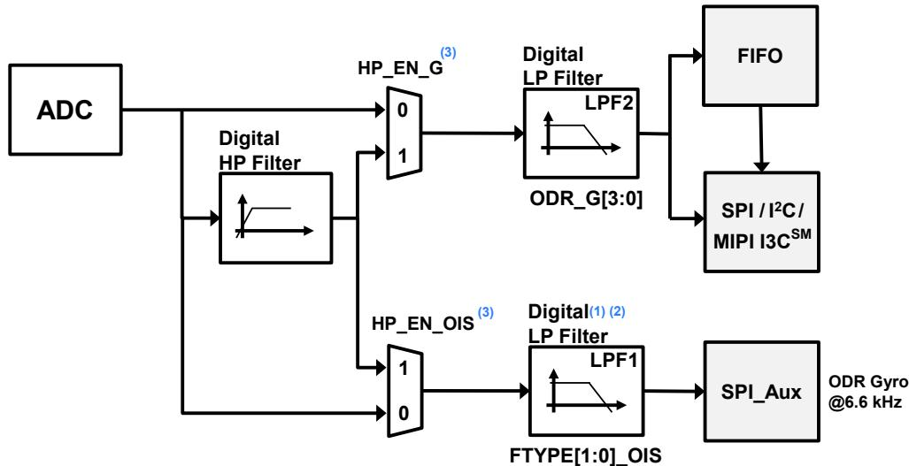
1. When Mode3/4 is enabled, the LPF1 filter is not available in the gyroscope UI chain.
