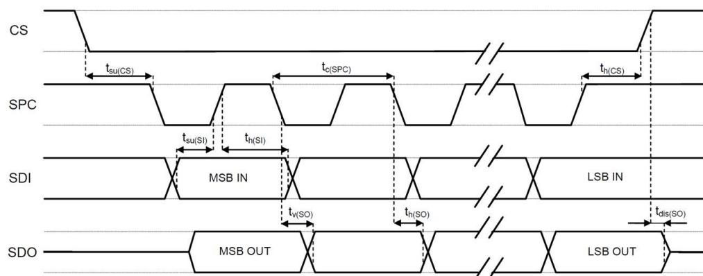
Note: Measurement points are done at  $0.2 \cdot Vdd\_IO$  and  $0.8 \cdot Vdd\_IO$  for both input and output ports.
