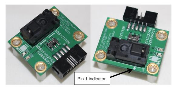
Please note the Pin 1 indicator: Ensure IC is placed in socket with Indicator in the Left Bottom position.
