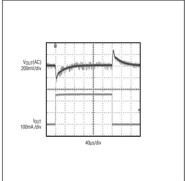
Figure 4. MAX17501G No Load to 250mA Load Transient
