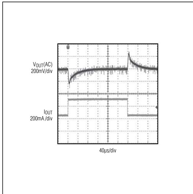
Figure 5. MAX17501G 250mA to 500mA Load Transient
