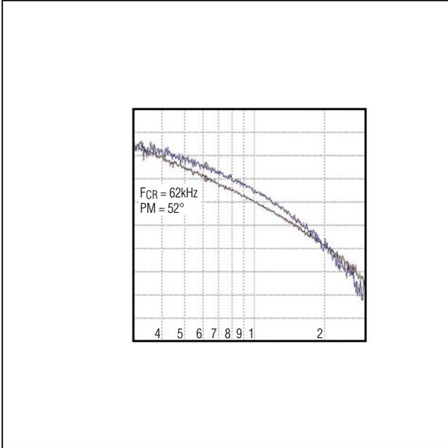
Figure 3. MAX17501G Full-Load Bode Plot ( $V_{IN} = 24V$ )
