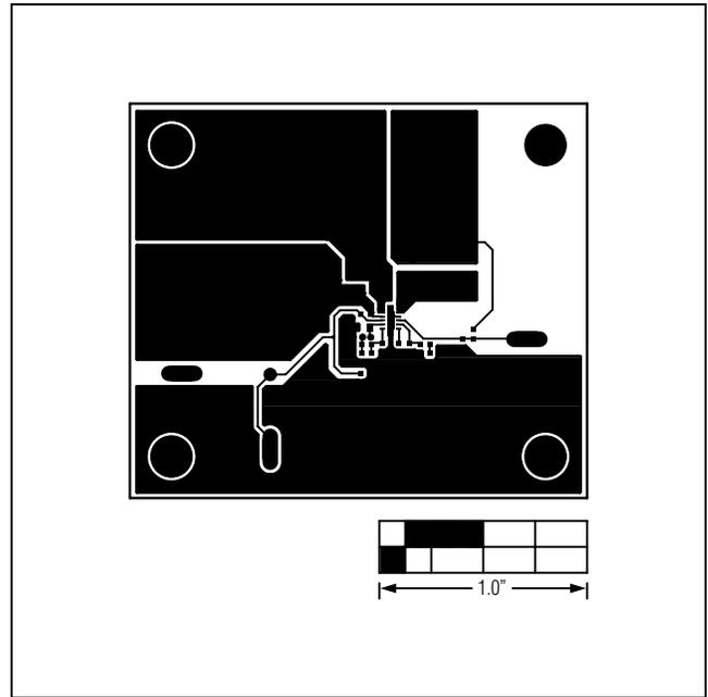
Figure 8. MAX17501G EV Kit PCB Layout—Component Side
