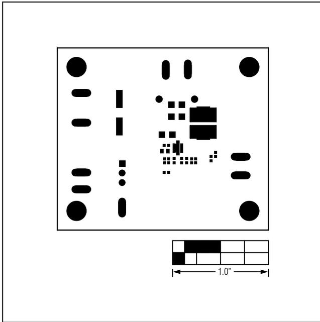
Figure 10. MAX17501G EV Kit PCB Layout—Top Solder Mask
