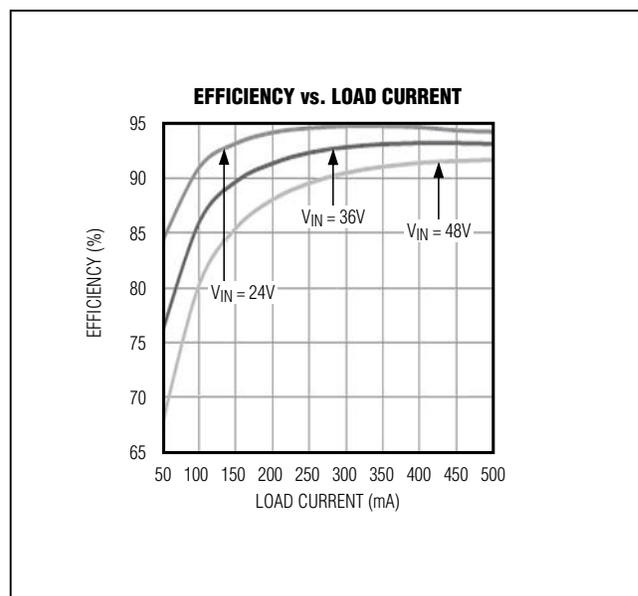
Figure 2. MAX17501G Efficiency
