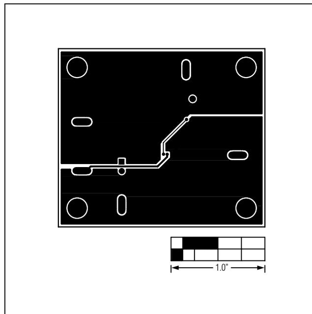
Figure 9. MAX17501G EV Kit PCB Layout—Solder Side
