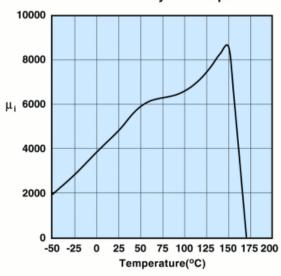
Measured on a 17/10/6mm toroid at 10kHz.
