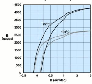
Measured on a 17/10/6mm toroid at 10kHz.
