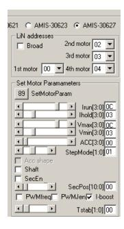
Give a position with the position slider and click the Set Position Command button. The motor should perform a positioning to the given position.
