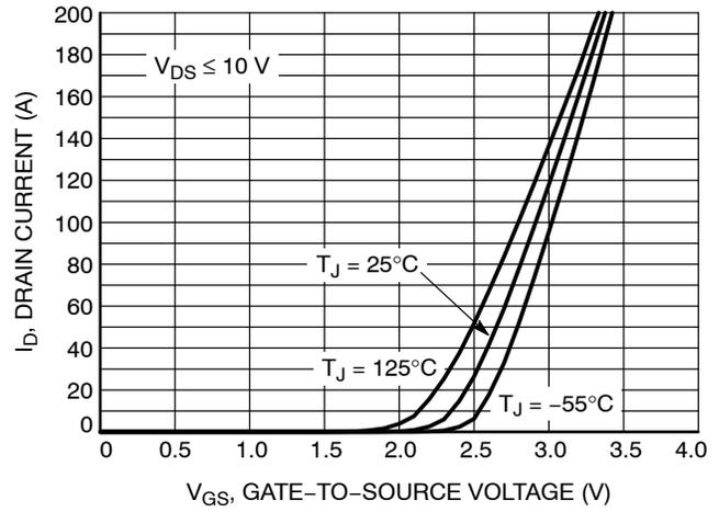
Figure 2. Transfer Characteristics
