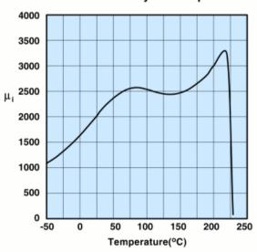
Measured on an 18/10/6mm toroid at 100kHz.
