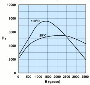
Measured on an 18/10/6mm toroid at 10kHz.
