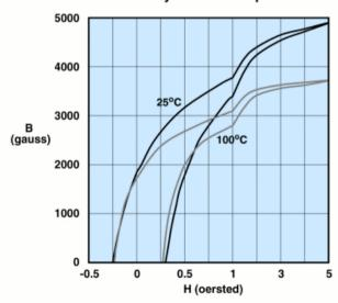
Measured on an 18/10/6mm toroid at 10kHz.
