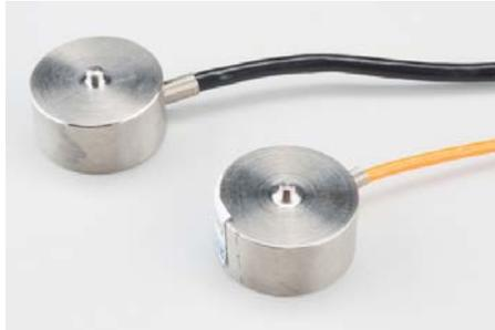
For smaller, push-button or disc load cells, you will want to make sure to screw in the disc to a bottom plate (or surface you are measuring force against), and center the beam, plate, or whatever else you are wishing to measure the force of onto the "button" on the top. Usually another plate with a hole is used to make sure whatever you are measuring is hitting the same spot on the load cell each time, but it is not necessary.
