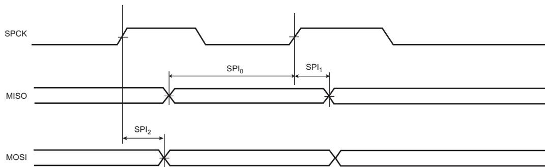
**Figure 41-21. SPI Master Mode with (CPOL = 0 and NCPHA = 1) or (CPOL = 1 and NCPHA = 0)**
