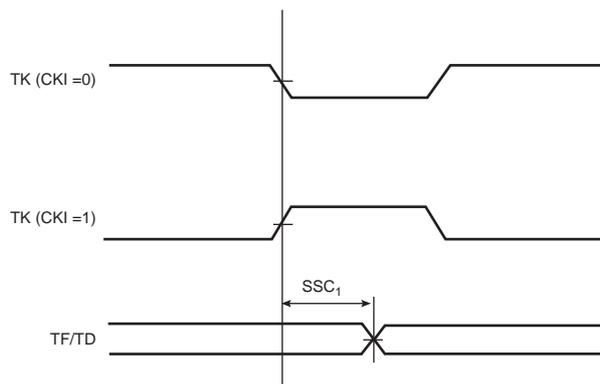
**Figure 41-26. SSC Transmitter, TK as Output and TF as Input**
