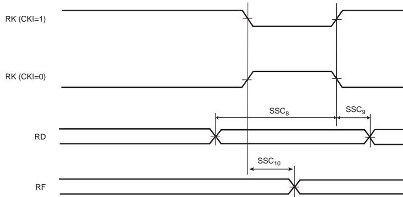
**Figure 41-30. SSC Receiver, RK and RF as Output**
