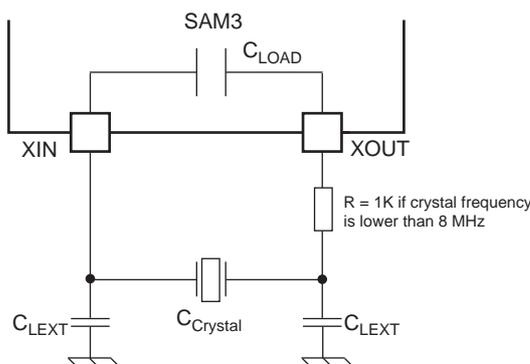
$$C_{LEXT} = 2 \times (C_{CRYSTAL} - C_{LOAD} - C_{PCB})$$
