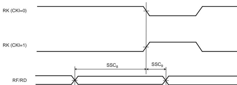
**Figure 41-29. SSC Receiver, RK as Input and RF as Output**
