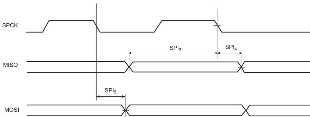
**Figure 41-22. SPI Slave Mode with (CPOL = 0 and NCPHA = 1) or (CPOL = 1 and NCPHA = 0)**
