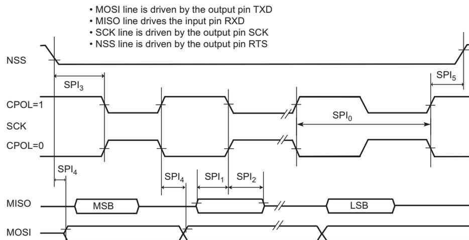
**Figure 41-36. USART SPI Slave Mode (Mode 1 or 2)**
