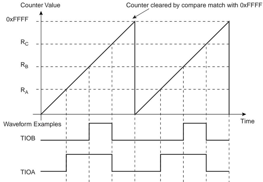
**Figure 34-8. WAVSEL= 00 with trigger**
