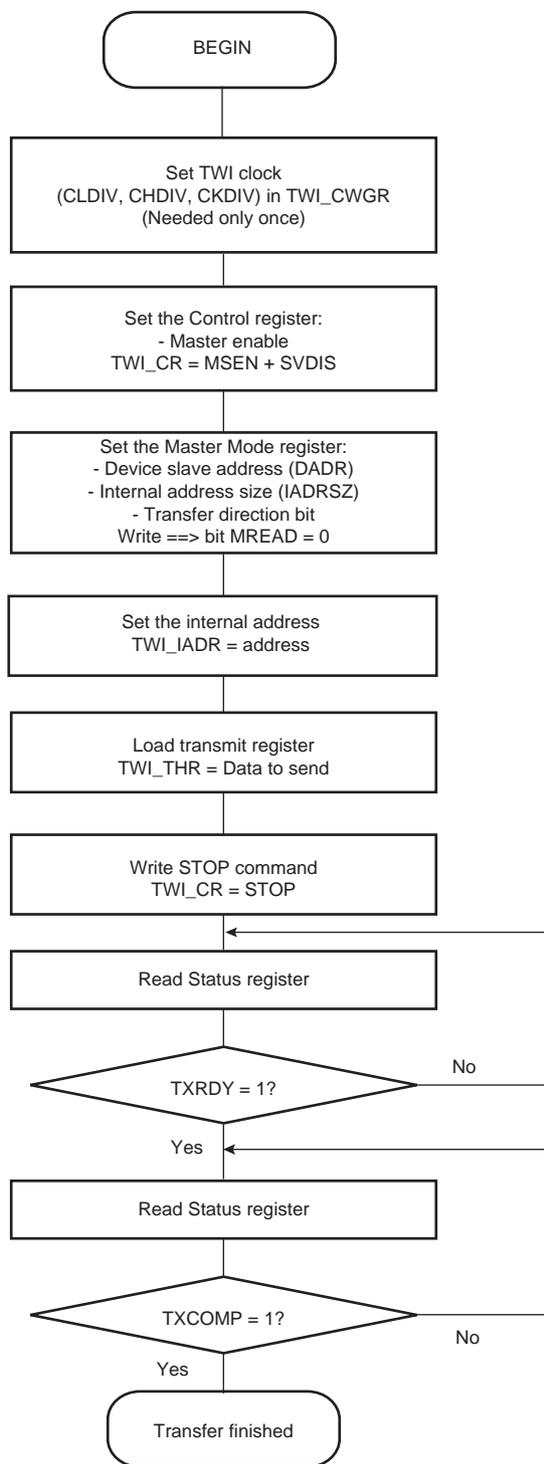
Figure 30-17. TWI Write Operation with Multiple Data Bytes with or without Internal Address
