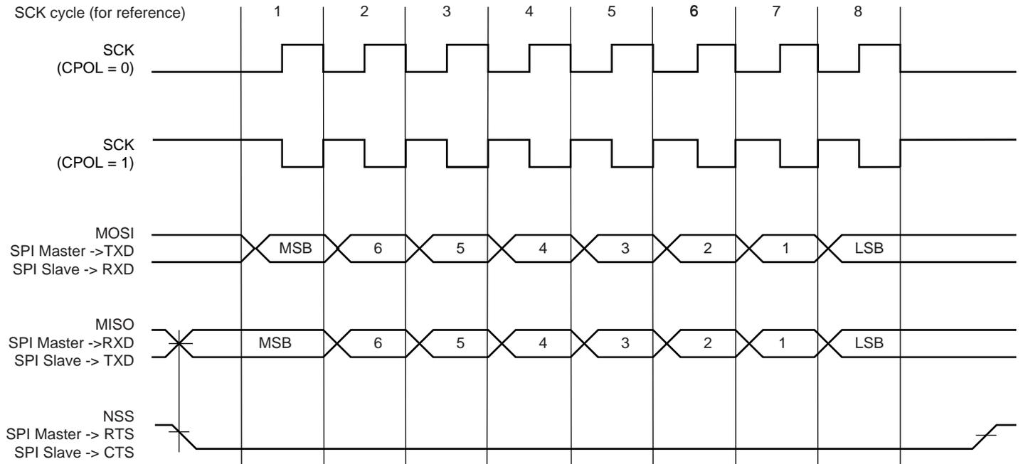
**Figure 33-39. SPI Transfer Format (CPHA=0, 8 bits per transfer)**
