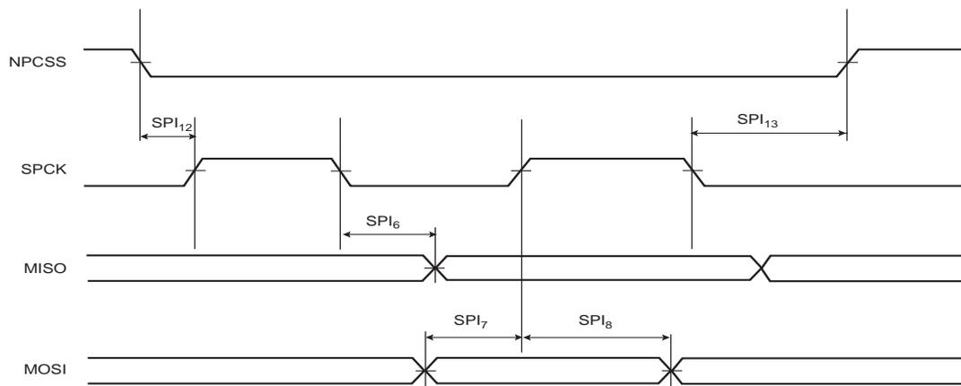
**Figure 41-23. SPI Slave Mode with (CPOL = NCPHA = 0) or (CPOL = NCPHA = 1)**
