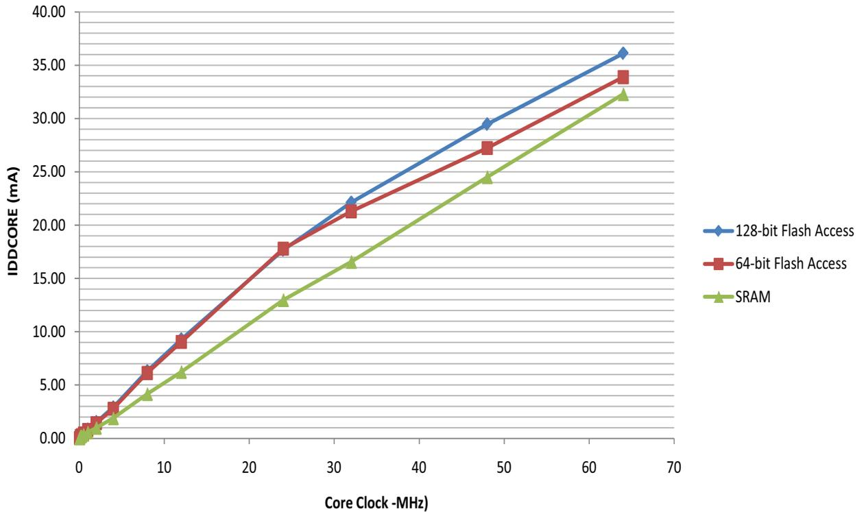
**Table 41-12. Active Power Consumption with VDDCORE @ 1.62V Running from Flash Memory or SRAM**
