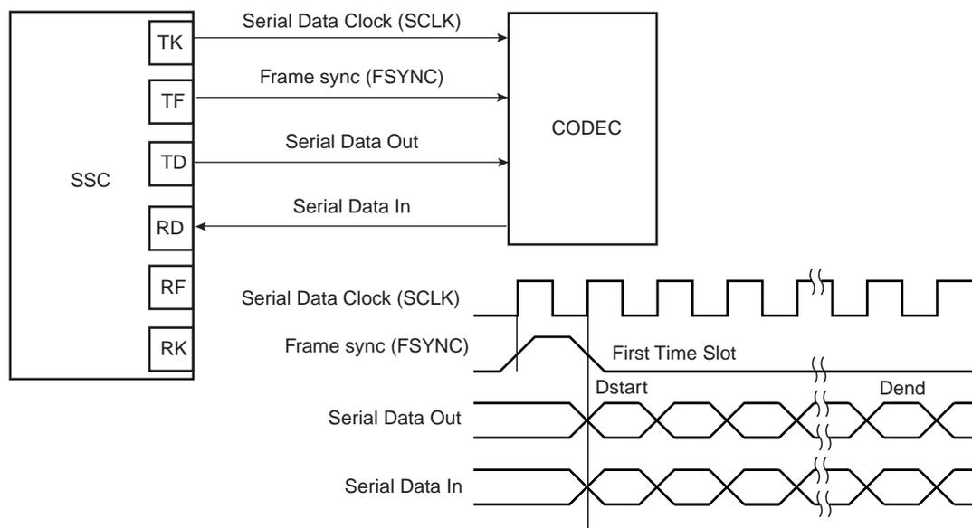
**Figure 29-19. Time Slot Application Block Diagram**
