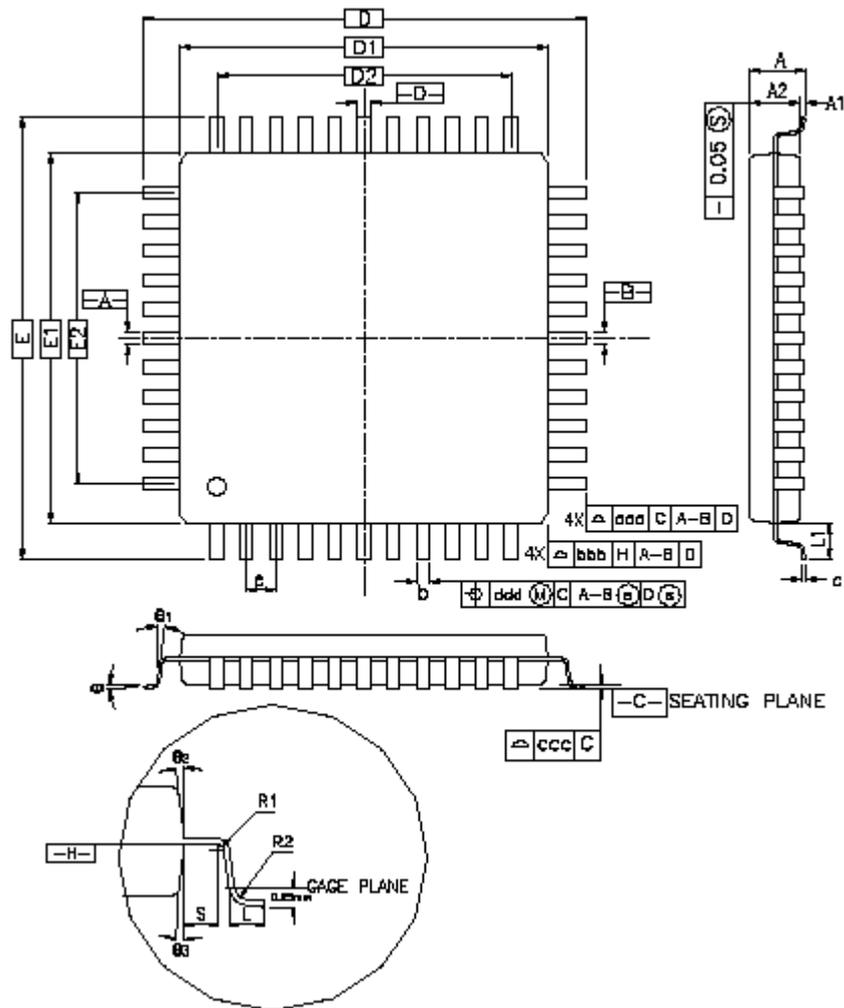
**Table 42-8. 64-lead LQFP Package Dimensions (in mm)**
