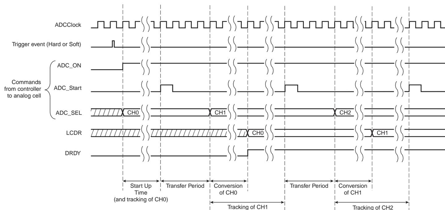
**Figure 39-3. Sequence of ADC conversions when Tracking time < Conversion time**
