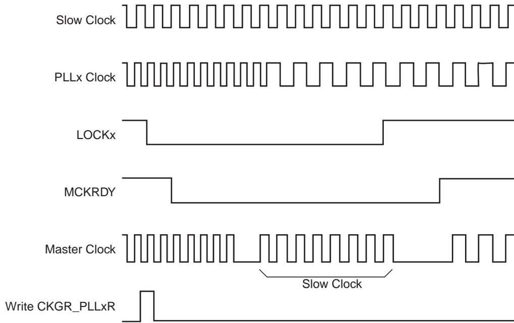
**Figure 26-8. Programmable Clock Output Programming**
