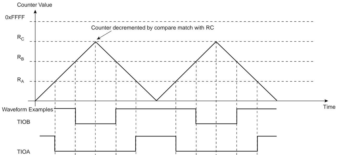
**Figure 34-14. WAVSEL = 11 With Trigger**
