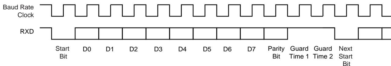
**Figure 33-32. T = 0 Protocol with Parity Error**
