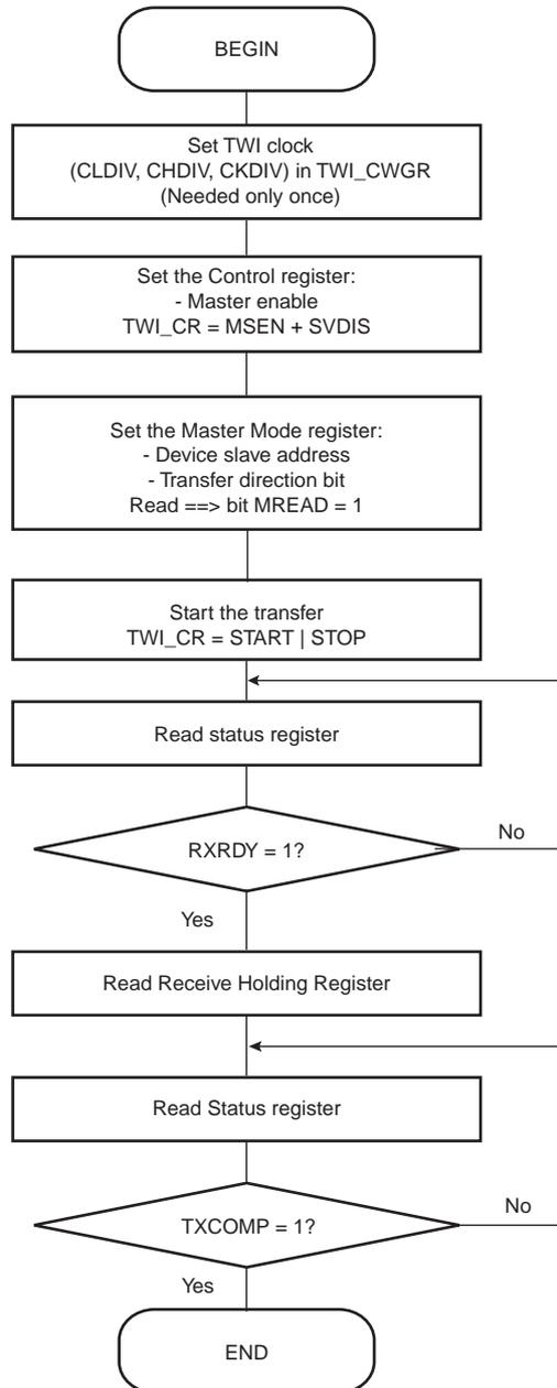
Figure 30-19. TWI Read Operation with Single Data Byte and Internal Address
