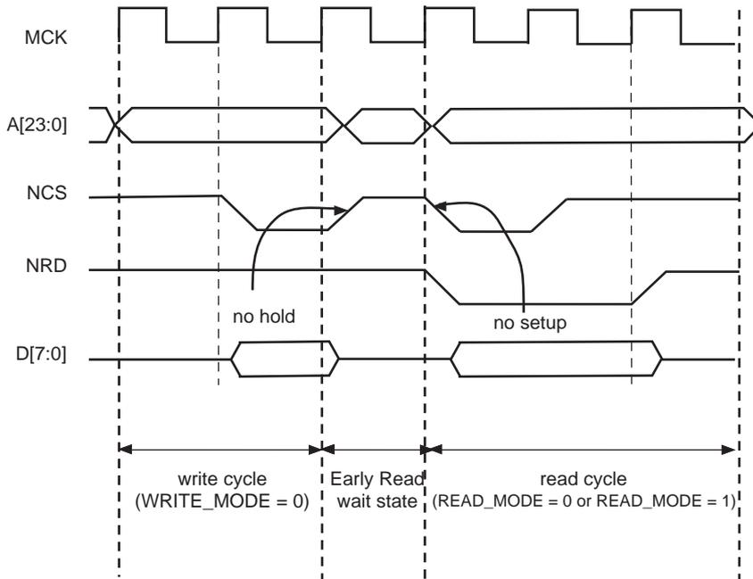
**Figure 23-16. Early Read Wait State: NWE-controlled Write with No Hold Followed by a Read with one Set-up Cycle**
