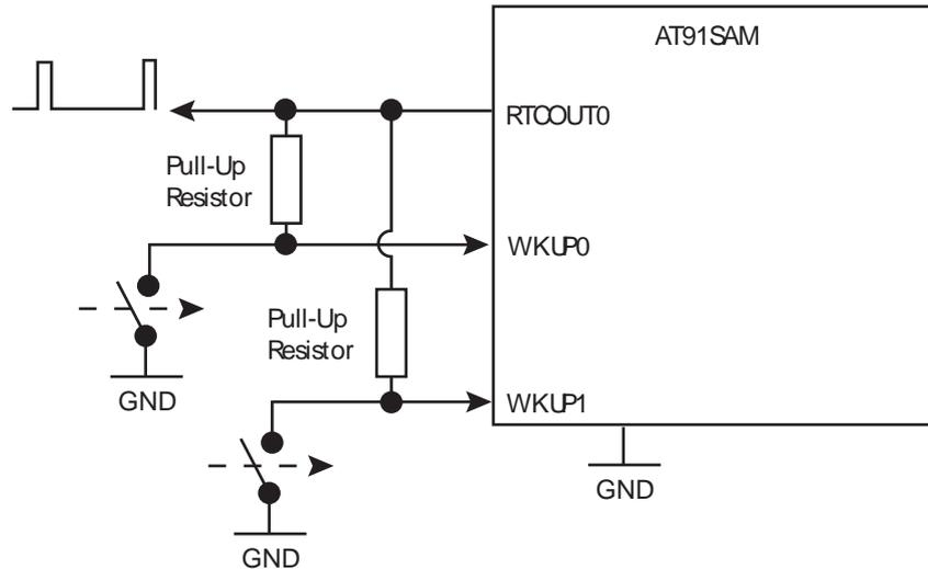
**Figure 16-6. Low Power Debouncer (Push-to-Break switch, pull-down resistors)**
