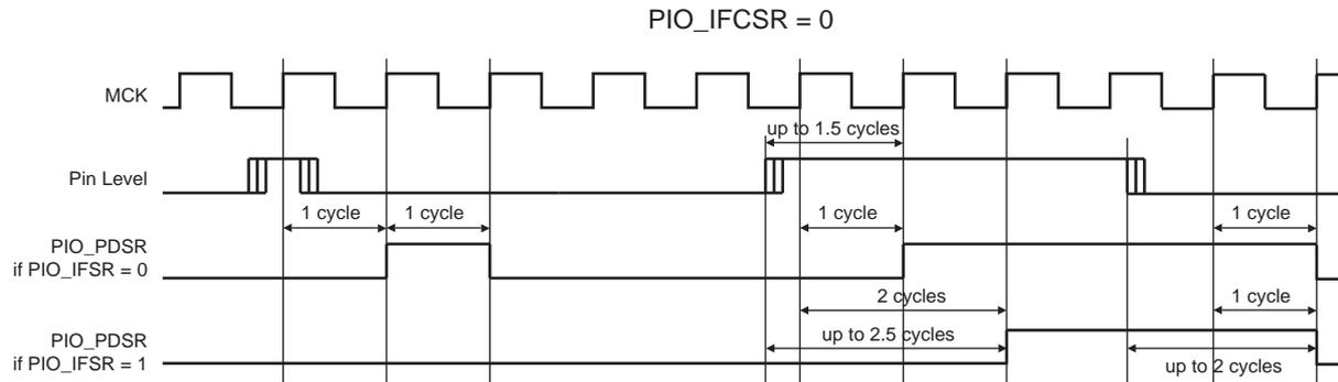
**Figure 28-6. Input Debouncing Filter Timing**
