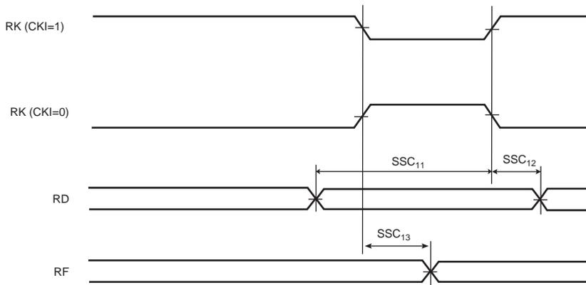
**Figure 41-31. SSC Receiver, RK as Output and RF as Input**
