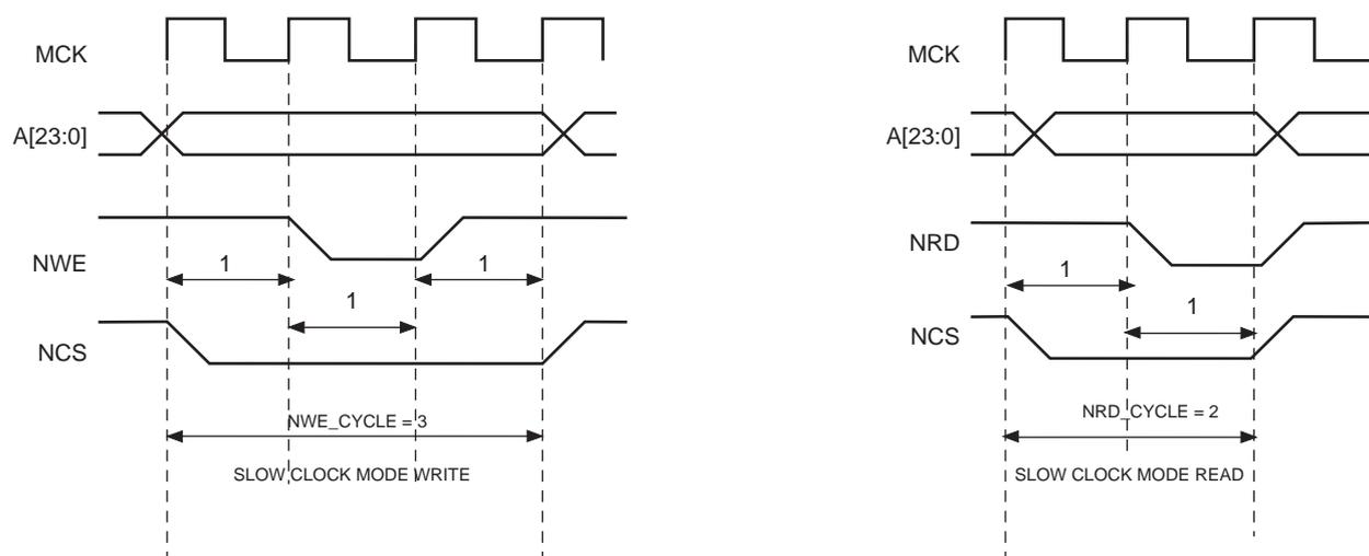
Table 23-4. Read and Write Timing Parameters in Slow Clock Mode
