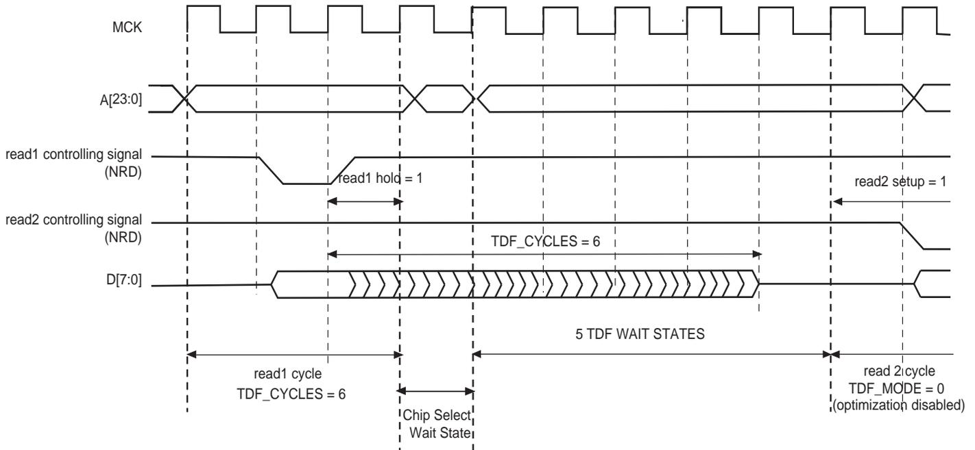
**Figure 23-21. TDF Mode = 0: TDF wait states between a read and a write access on different chip selects**
