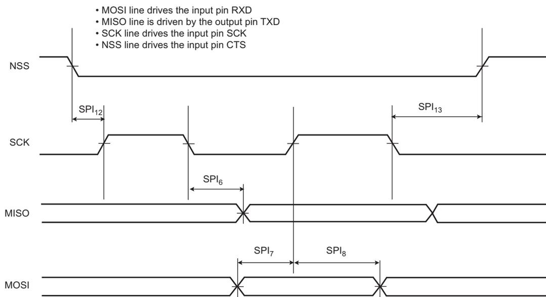
Figure 41-37. USART SPI Slave Mode (Mode 0 or 3)
