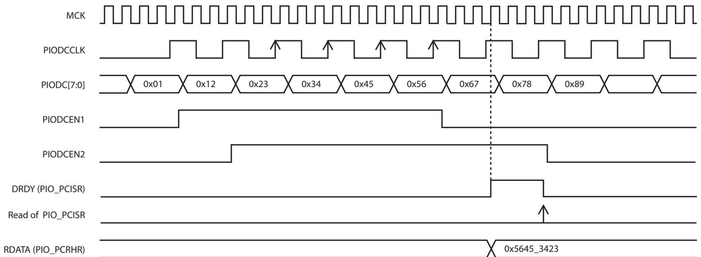
**Figure 28-11. Parallel Capture Mode Waveforms (DSIZE=2, ALWYS=1, HALFS=0)**
