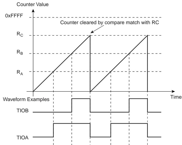
**Figure 34-10. WAVSEL = 10 With Trigger**
