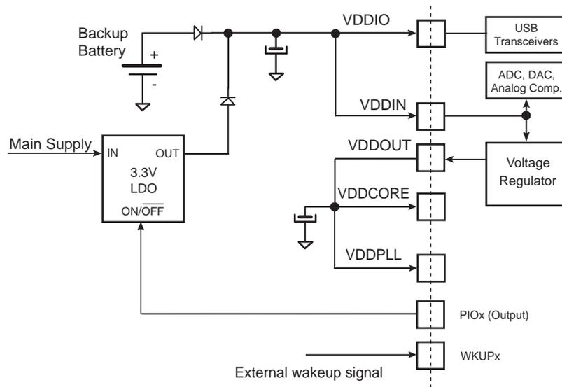
Note: The two diodes provide a “switchover circuit” (for illustration purpose) between the backup battery and the main supply when the system is put in backup mode.
