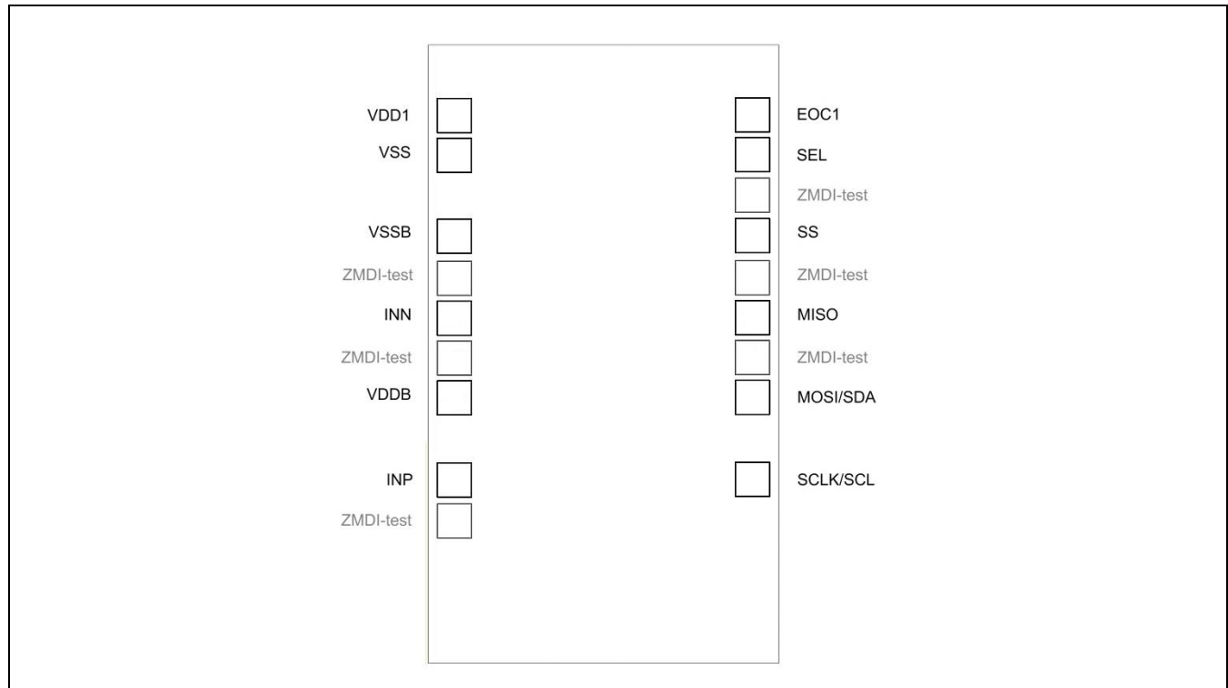
Figure 4.1 ZSSC3036 Pad Assignments
