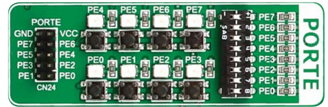
Figure 6-1: I/O group contains PORT header, tri-state pull up/down DIP switch, buttons and LEDs all in one place
