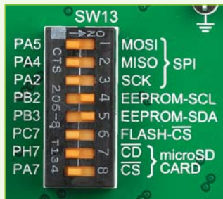
Figure 23-2: Activate SW13.4 and SW13.5 switches to enable pull-up resistors in I 2 C lines of Serial EEPROM.
