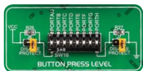
Figure 6-5: Button press level DIP switch (tri-state)
