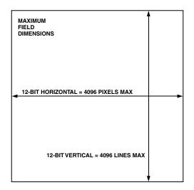
Figure 6. Vertical and Horizontal Counters
