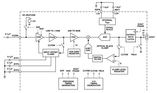
Figure 36. AFE Block Diagram
