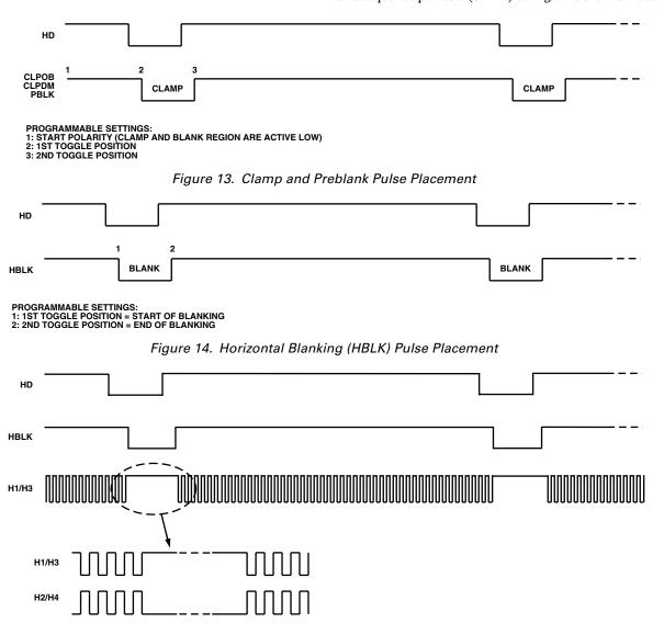
THE POLARITY OF H1 DURING BLANKING IS PROGRAMMABLE (H2 IS OPPOSITE POLARITY OF H1)
