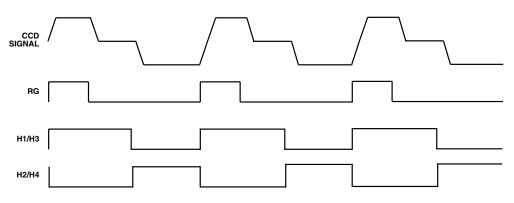
USING THE SAME TOGGLE POSITIONS FOR H1 AND H3 GENERATES STANDARD 2-PHASE H-CLOCKING.
