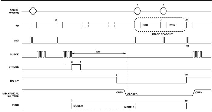
Figure 35. Exposure and Readout of Interlaced Frame
