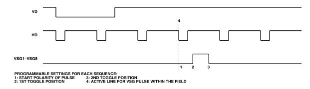
Figure 29. Vertical Sensor Gate Pulse Placement
