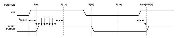
PIXEL CLOCK PERIOD IS DIVIDED INTO 48 POSITIONS. PROVIDING FINE EDGE RESOLUTION FOR HIGH SPEED CLOCKS. THERE IS A FIXED DELAY FROM THE CLI INPUT TO THE INTERNAL PIXEL PERIOD POSITIONS (t<sub>CLIDLY</sub> = 6ns TYP).
