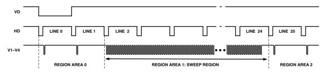
Figure 26. Example of Sweep Region for High Speed Vertical Shift
