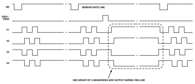
Figure 25. Example of Second Sequences During Sensor Gate Line
