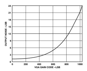
TPC 6. AD9895 Output Noise vs. VGA Gain
