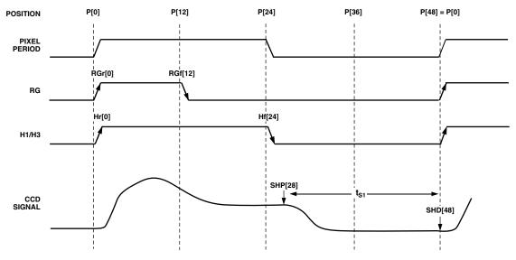
NOTES ALL SIGNAL EDGES ARE FULLY PROGRAMMABLE TO ANY OF THE 48 POSITIONS WITHIN ONE PIXEL PERIOD. DEFAULT POSITIONS FOR EACH SIGNAL ARE SHOWN.
