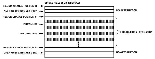
WHEN THE VTPALT REGISTER IS LOW (NO ALTERNATION), ONLY THE FIRST LINES ARE USED.
