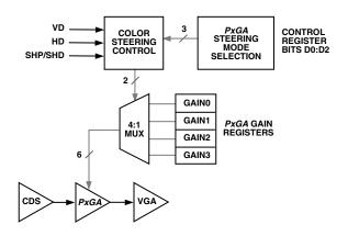
Figure 37. PxGA Block Diagram
