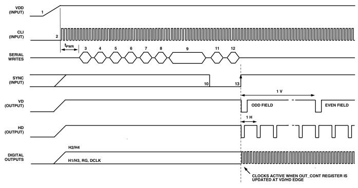
Figure 42. Recommended Power-Up Sequence and Synchronization, Master Mode
