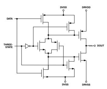
Figure 2. Digital Data Outputs
