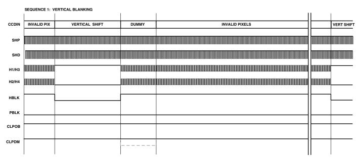
CLPDM PULSE MAY BE USED DURING HORIZONTAL DUMMY PIXELS IF THE H-CLOCKS ARE USED DURING VERTICAL BLANKING.
