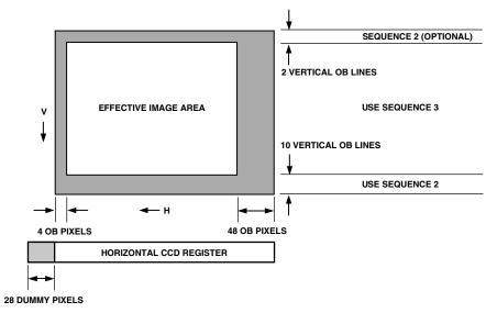
Figure 45. Example CCD Configuration
