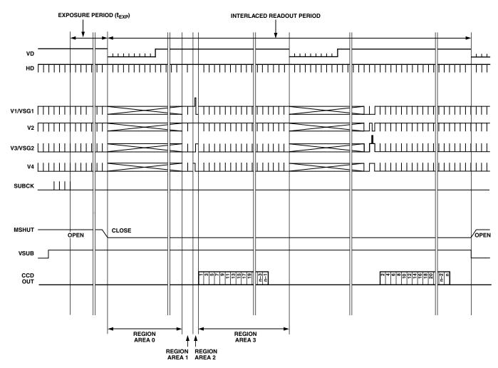
Figure 49. Vertical Timing Example—Separate Regions
