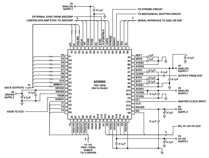
Figure 50. AD9891/AD9895 Typical Circuit Configuration
