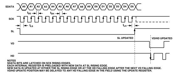
Figure 52. Serial Write Operation
