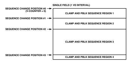
UP TO FOUR INDIVIDUAL HORIZONTAL CLAMP AND BLANKING REGIONS MAY BE PROGRAMMED WITHIN A SINGLE FIELD, USING THE SEQUENCE CHANGE POSITIONS.
