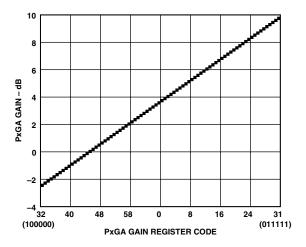
Figure 40. PxGA Gain Curve
