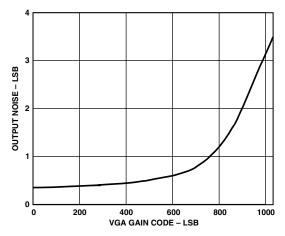
TPC 3. AD9891 Output Noise vs. VGA Gain
