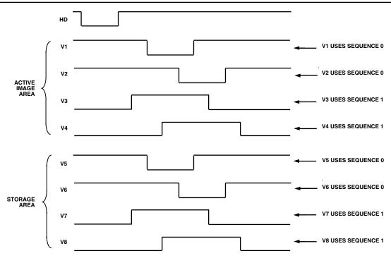
Figure 28. Example of Frame Transfer CCD Mode using V1-V8
