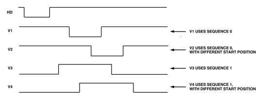
Figure 19. Example of Separate V1–V4 Signals Using Two Individual Sequences
