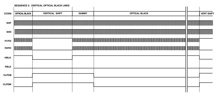
Figure 47. Horizontal Sequences During Vertical Optical Black Pixels
