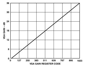
Figure 41. VGA Gain Curve (PxGA not included)
