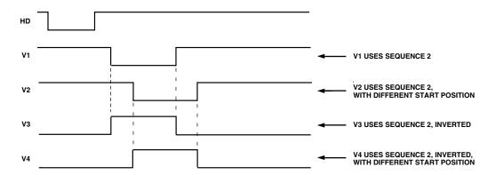
Figure 20. Example of Inverted V1-V4 Signals Using One Individual Sequence with Inversion
