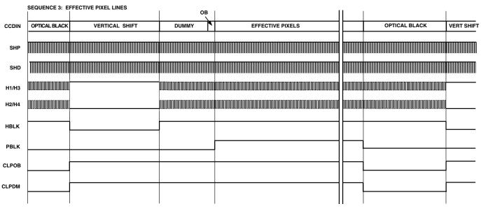
Figure 48. Horizontal Sequences During Effective Pixels
