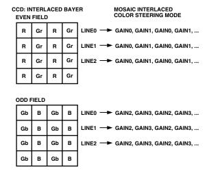
Figure 38b. CCD Color Filter Example: Interlaced
