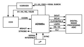
Figure 5. Typical System Block Diagram, Master Mode Alternatively, the AD9891/AD9895 may be operated in Slave Mode, in which the VD and HD are provided externally from the image processor. In this mode, all AD9891/AD9895 timing will be synchronized with VD and HD.
