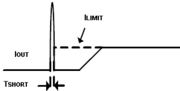
Figure 2. Response Time to Short Circuit Waveform
