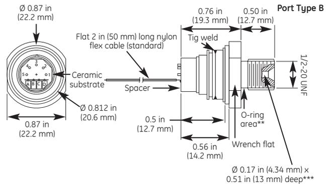
\*Uses o-ring 0.66 in ID x 0.039 in (16076 mm x 1 mm) cross section.
