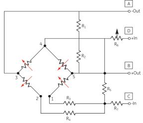
Constant voltage schematic diagram
