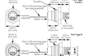
\*Uses o-ring 0.66 in ID  $\times$  0.039 in (16076 mm  $\times$  1 mm) cross section. \*\*Uses 2-013 per ISO 360 1/1 o-ring for outside seal. \*\*\*Uses 2-003 per ISO 360 1/1 o-ring for inside seal.
