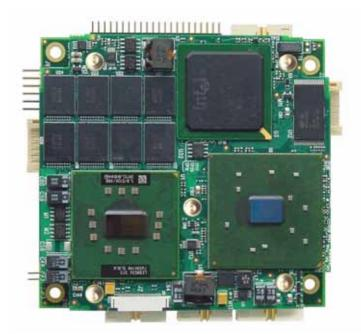
The CPU-1484 is an embedded RoHS compliant board based on two modules: a mezzanine CPU module combined with a PC/104-Plus form factor carrier.
