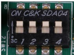
The DIP test checks the DIP switch, SW12 operation. To complete the test, push all four switches into the ON position.
