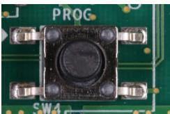
To run the Board Self Test again, press SW4 (PROG).
