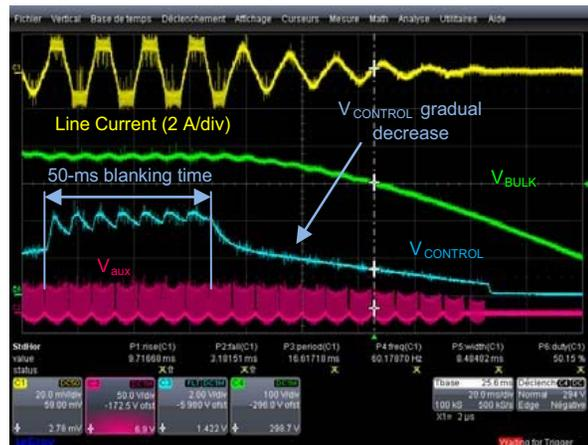
c) Abrupt line drop (90 V to 70 V)
