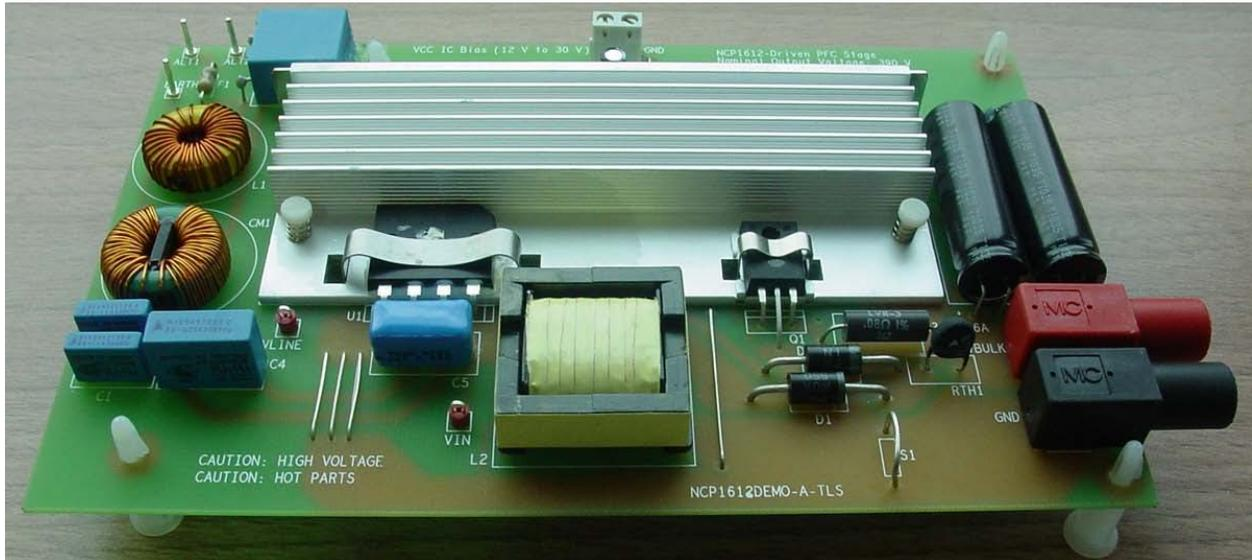
Figure 1. A Slim Board (Height < 13 mm)
