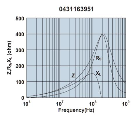
Impedance, reactance, and resistance vs. frequency.
