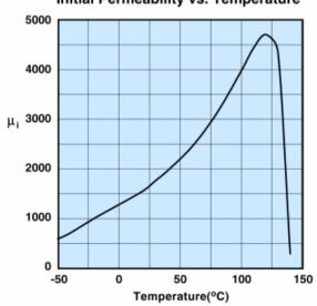
Measured on a 17/10/6mm toroid at 100kHz.
