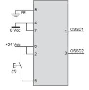
(1) Restart With External Device Monitoring (EDM) feedback loop
