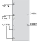
With External Device Monitoring (EDM) feedback loop
