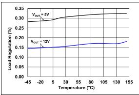
FIGURE 2-2: LDO Load Regulation vs. Temperature.
