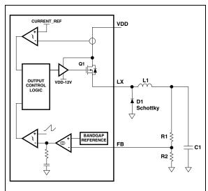
Start with an R2 value of 10 k $\Omega$  to 51 k $\Omega$  to minimize current through the divider.
