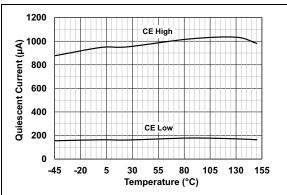
FIGURE 2-14: Quiescent Current vs. Temperature (MCP8026).
