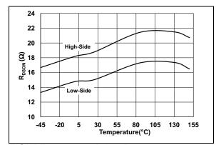
**FIGURE 2-16:** Driver  $R_{DSON}$  vs. Temperature.
