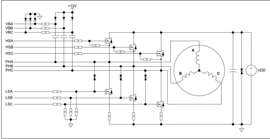
FIGURE 5-3: Overvoltage Protection.
