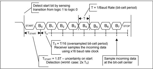
FIGURE 4-3: DE2 Packet Timing.
