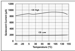
**FIGURE 2-13:** Quiescent Current vs. Temperature (MCP8025).
