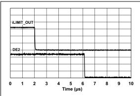
FIGURE 2-3: I<sub>LIMIT\_OUT</sub> Low to DE2 Message Delay.
