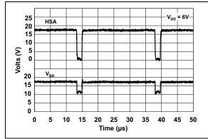
FIGURE 2-4: Bootstrap Voltage @ 92% Duty Cycle.
