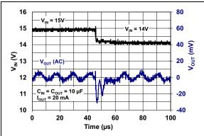
FIGURE 2-9: - Falling V<sub>DD</sub>.
