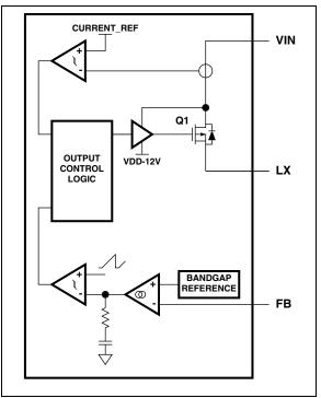
**FIGURE 4-1:** SMPS Functional Block Diagram.
