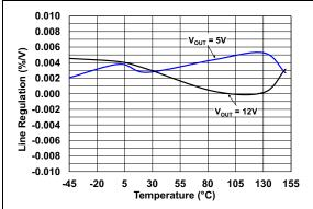
FIGURE 2-1: LDO Line Regulation vs. Temperature.
