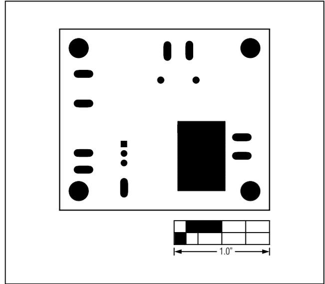
Figure 11. MAX17501H EV Kit PCB Layout—Bottom Solder Mask
