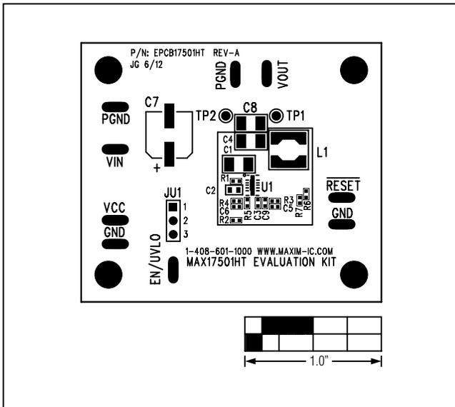
Figure 7. MAX17501H EV Kit Component Placement Guide—Component Side
