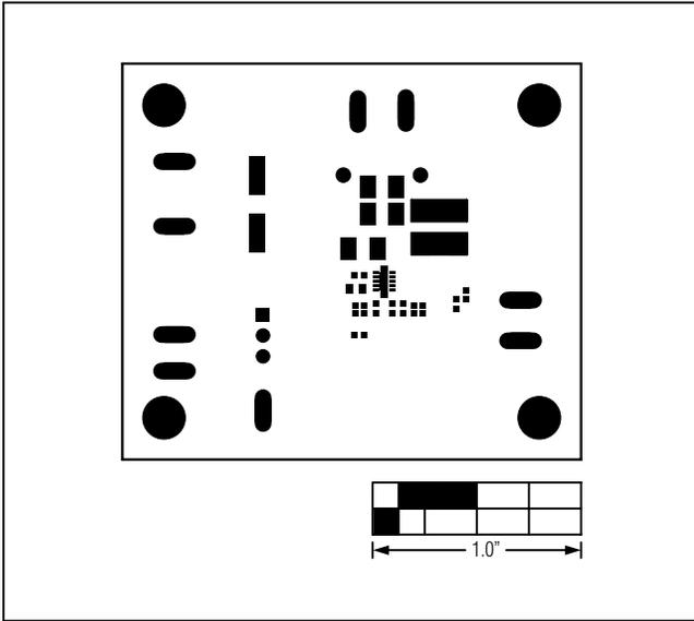
Figure 10. MAX17501H EV Kit PCB Layout—Top Solder Mask
