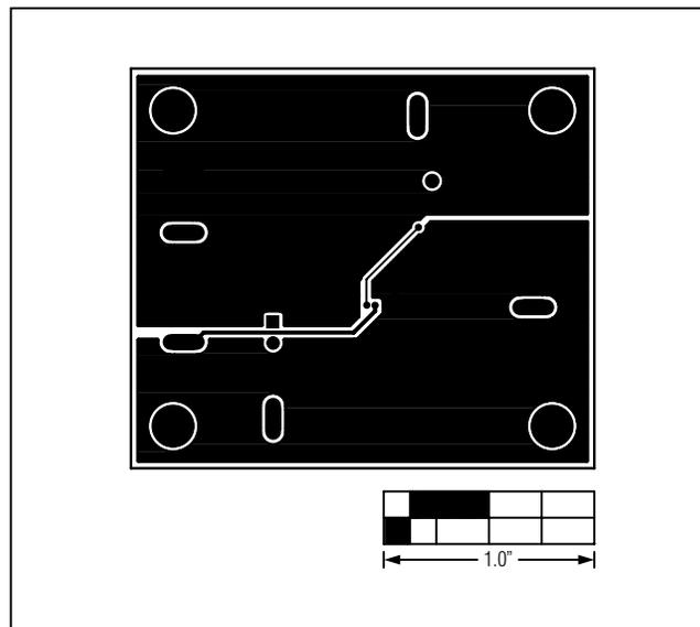
Figure 9. MAX17501H EV Kit PCB Layout—Solder Side
