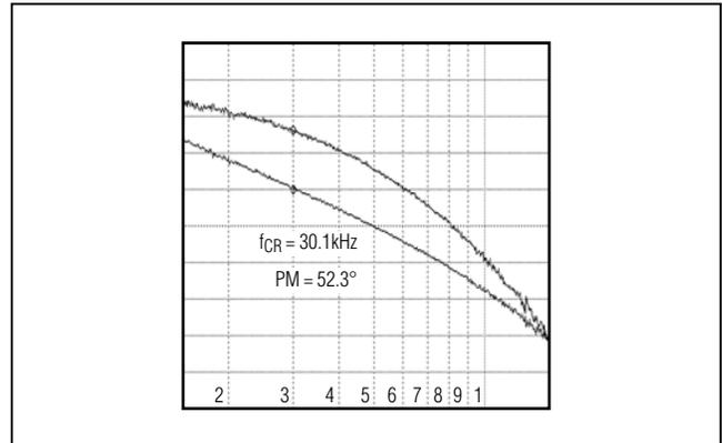
Figure 3. MAX17501H Full-Load Bode Plot (VIN = 24V)
