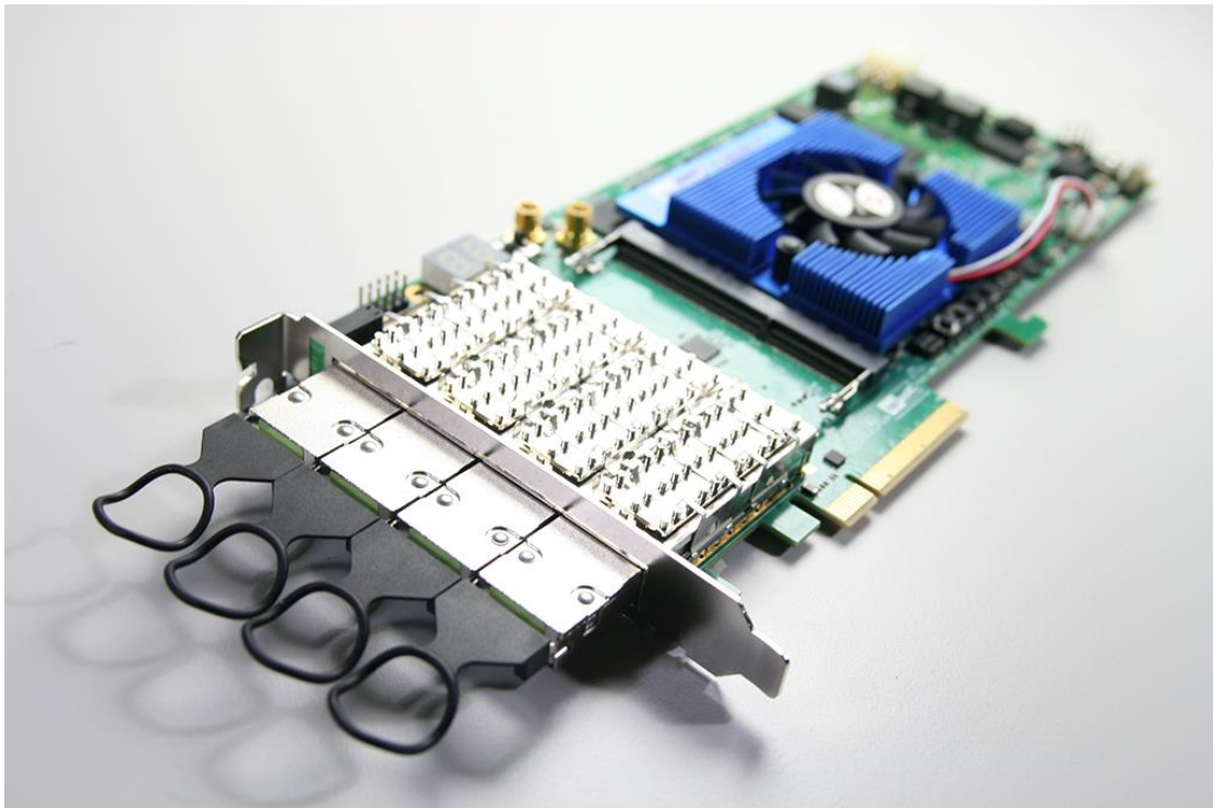
Figure 8-4 Four QSFP+ Loopback Fixtures Installed
