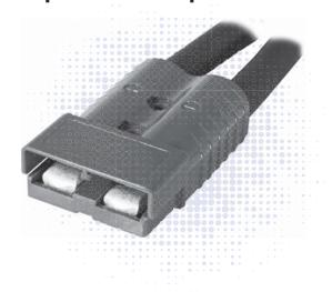
The SB®350 is the largest connector in the series with power capabilities up to 450 amps with 4/0 AWG wire and 500 amps with a 350 mcm wire. Wires ranging from #1/0 (53.5 mm²) to 350 mcm (150 mm²) fit into the one piece housing available in standard PC or a chemical resistant PBT/PC blend. Silver plated wire or busbar contacts minimize electrical resistance while offering supreme durability and reliability.
