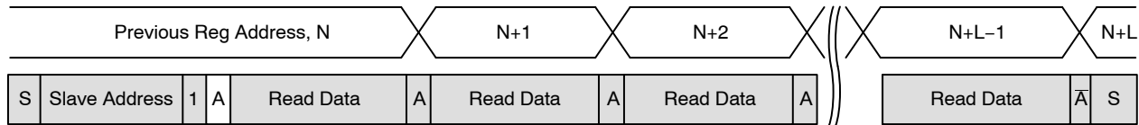
Figure 23. Sequential READ, Start from Current Location
