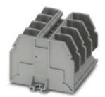
Feed-through terminal block with bolt connection method, cross section: 0.1 - 10 mm<sup>2</sup>, AWG: 26 - 8, width 13 mm. color: gray
