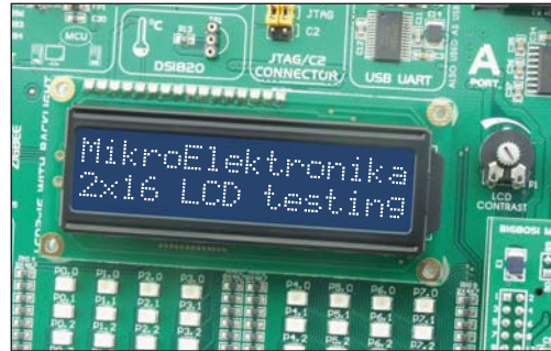
Figure 18-2: Alphanumeric 2x16 LCD display
