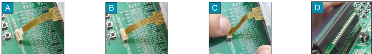
Figure 20-3: Connecting touch panel
