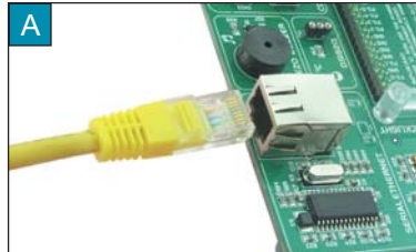
Figure 4-2: Connecting ethernet cable
