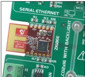
Figure 10-1: MRF24J40MA ZigBee module
