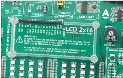
Figure 18-1: Connector for alphanumeric LCD display
