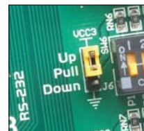
Figure 21-3: J9 in pull-up position
