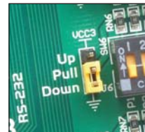
Figure 21-2: J9 in pull-down position
