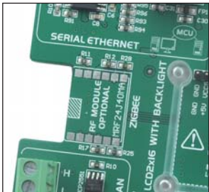
Figure 10-2: Connector for ZigBee module
