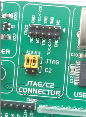
Figure 3-3: Connector for programmer
