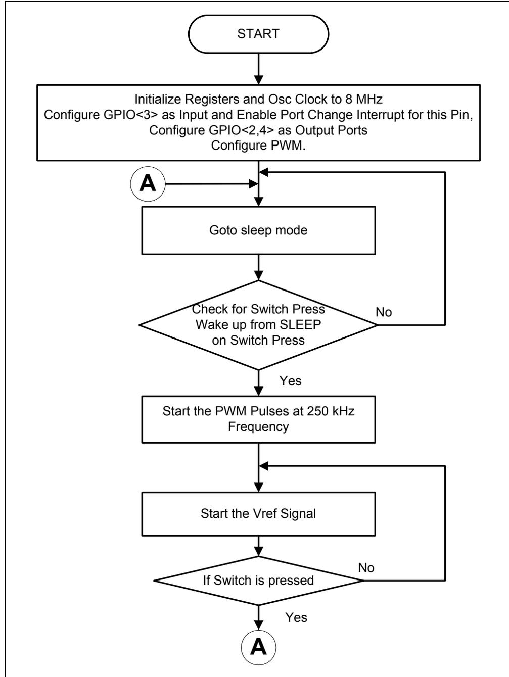
**FIGURE C-1:** *Firmware Flowchart.*
