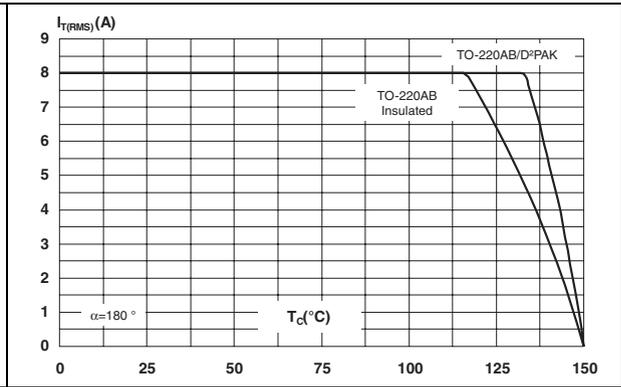
Figure 3. On-state rms current versus ambient temperature
