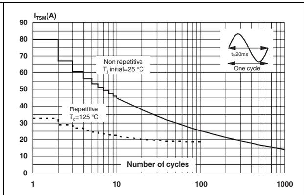
Figure 7. Non-repetitive surge peak on-state current for a sinusoidal pulse with
