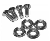
The 1421 screw provides a standard 0.625" rack screws length with 10-32 threads. The screw itself features a slotted oval head and has a nickel plate finish. The steel cup washers have an outside diameter of 0.60".
