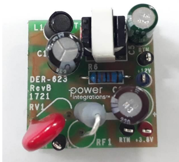
Figure 1 – Populated Circuit Board Photograph, Top.
