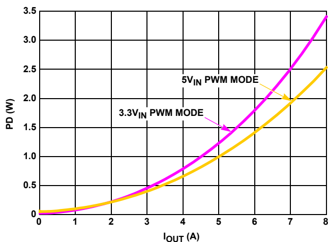
FIGURE 8. POWER DISSIPATION vs LOAD (1MHz, V_{OUT} = 1.8\text{V} )
