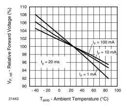
Fig. 4 - Relative Forward Voltage vs. Ambient Temperature
