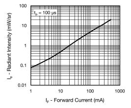
Fig. 5 - Radiant Intensity vs. Forward Current
