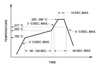
Fig. 9 - Lead (Pb)-free Reflow Solder Profile acc. J-STD-020
