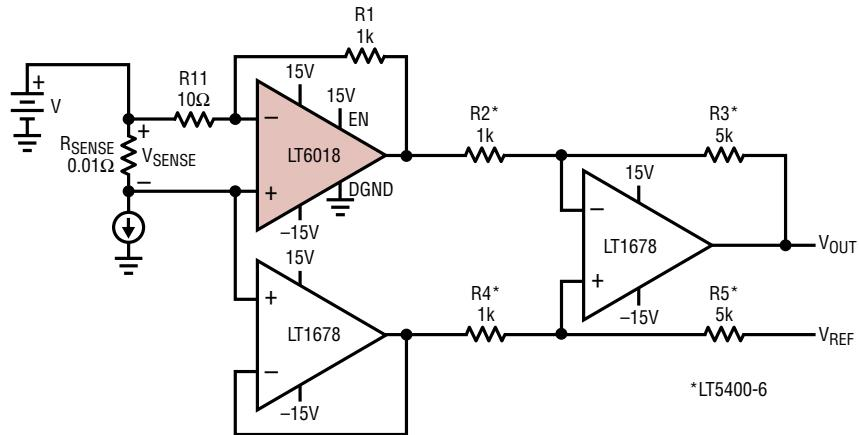
THE LT6018 IN THIS CIRCUIT PROVIDES LOW NOISE, LOW DISTORTION AMPLIFICATION OF A SMALL SENSE VOLTAGE DERIVED FROM A LOW IMPEDANCE SOURCE ACROSS A WIDE INPUT COMMON MODE RANGE.
