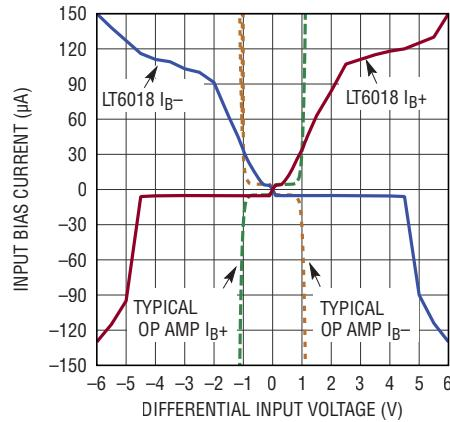
Figure 4. Typical Op Amp vs LT6018 Input Protection
