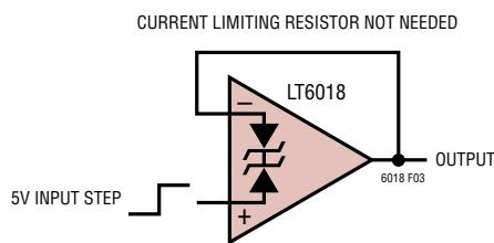
Figure 3. LT6018 Series Zener Diode Input Protection
