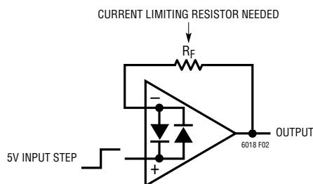
Figure 2. Typical Op Amp Diode Input Protection
